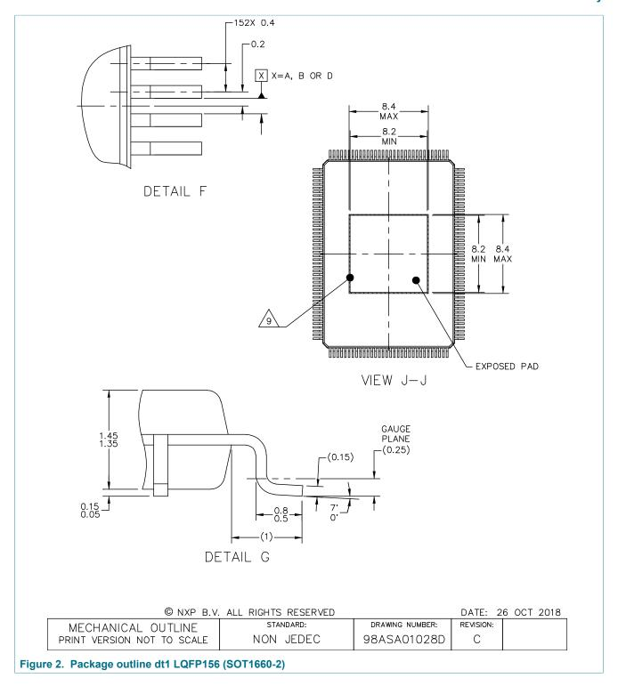
HLQFP156, plastic, thermal enhanced low profile quad flat package; 156 terminals; 0.4 mm pitch; 14 mm x 20 mm x 1.4 mm body
