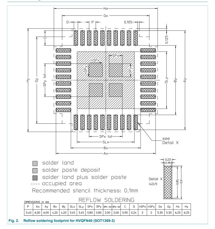
plastic thermal enhanced very thin quad flat package; no leads; 40 terminals; body 5 mm x 5 mm x 0.85
