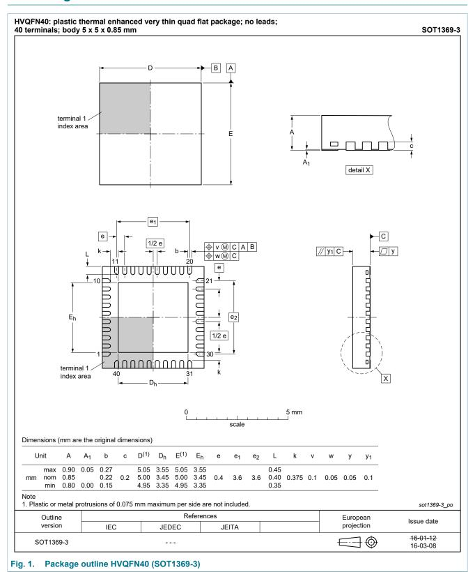
plastic thermal enhanced very thin quad flat package; no leads; 40 terminals; body 5 mm x 5 mm x 0.85 mm
