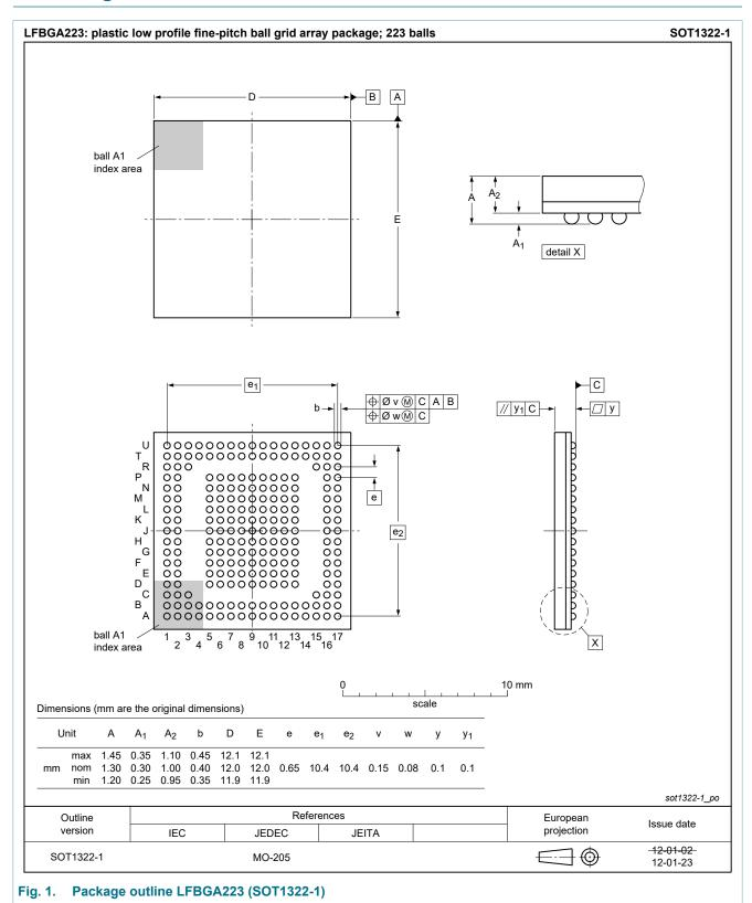
plastic low profile fine-pitch ball grid array package; 223 balls, 0.65 mm pitch, 12 mm x 12 mm x 1.3 mm body
