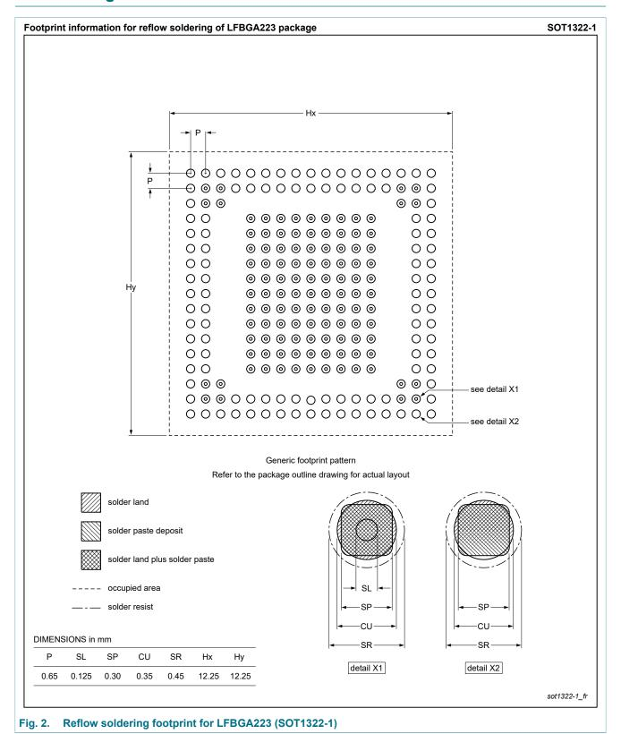
plastic low profile fine-pitch ball grid array package; 223 balls, 0.65 mm pitch, 12 mm x 12 mm x 1.3 mm body
