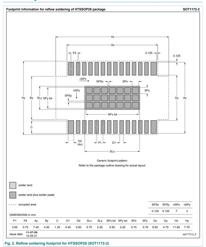
plastic thermal enhanced thin shrink small outline package; 28 leads; body width 4.4 mm; lead pitch 0.65 mm; exposed die pad
