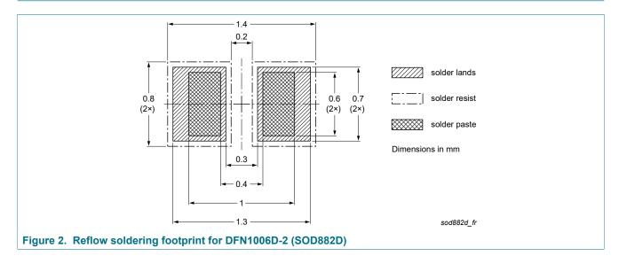
plastic, leadless ultra small plastic package; 2 terminals; 0.65 mm pitch; 1 mm x 0.6 mm x 0.4 mm body
