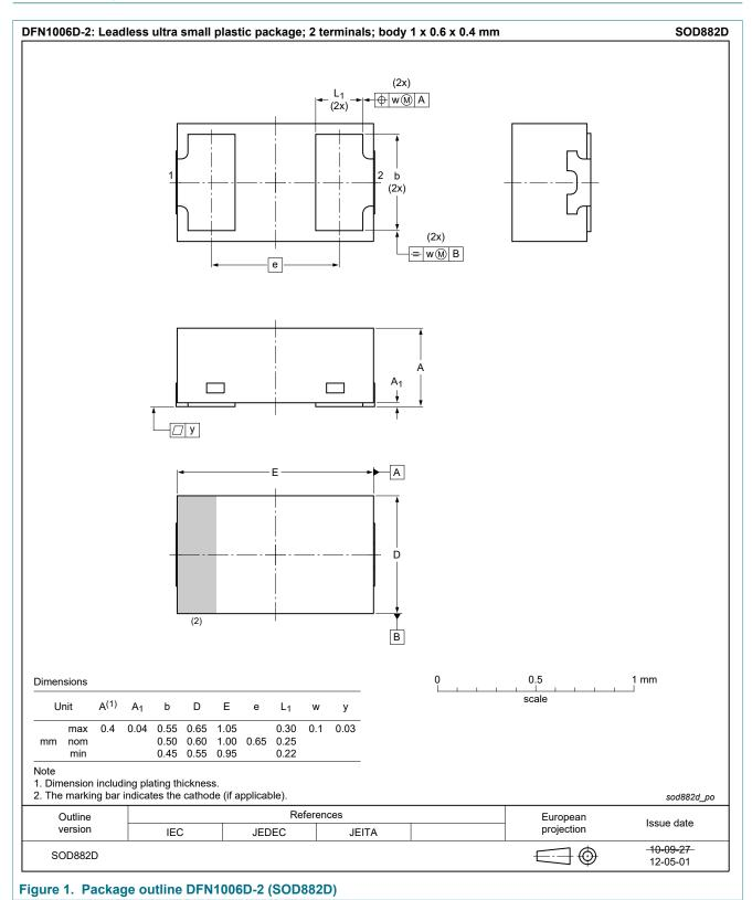
plastic, leadless ultra small plastic package; 2 terminals; 0.65 mm pitch; 1 mm x 0.6 mm x 0.4 mm body
