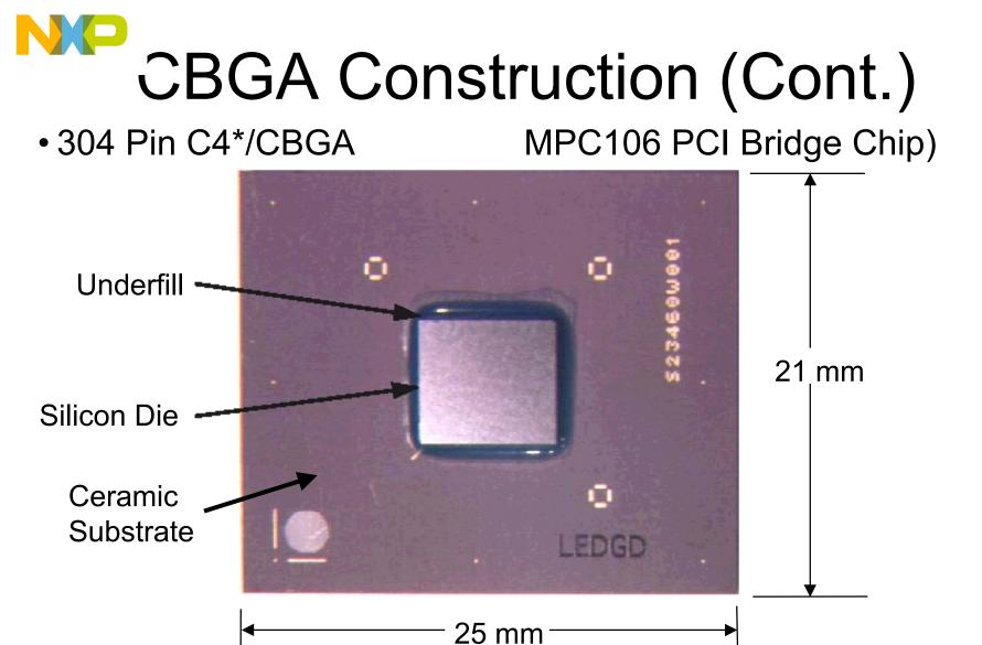
\* C4 = IBM Developed <u>Controlled</u> <u>Collapse</u> <u>Chip</u> <u>Conne</u>
