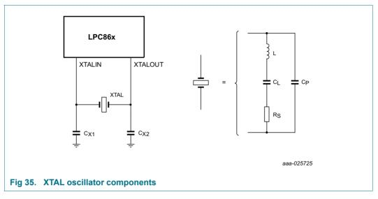
For best results, it is very critical to select a matching crystal for the on-chip oscillator. Load capacitance (CL), series resistance (RS), and drive level (DL) are important parameters to consider while choosing the crystal. After selecting the proper crystal, the external load capacitor  $C_{X1}$  and  $C_{X2}$  values can also be generally determined by the following expression:
