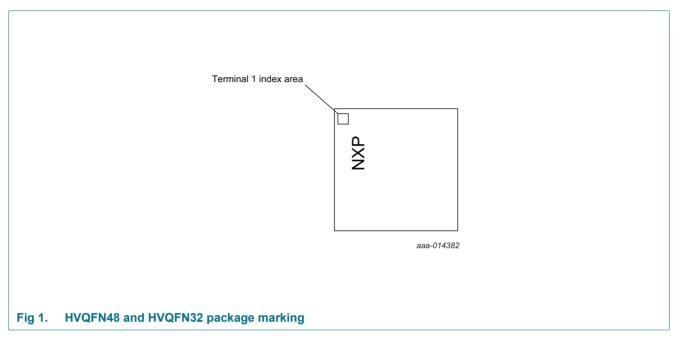
The LPC86x HVQFN48 package has the following top-side marking:
