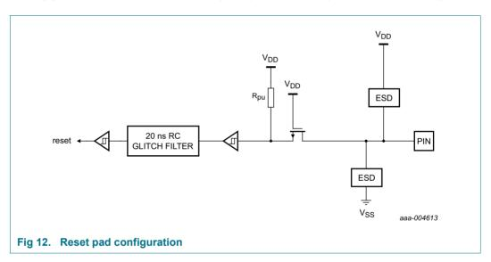
In deep power-down mode, an external pull-up resistor is required on the RESET pin.
