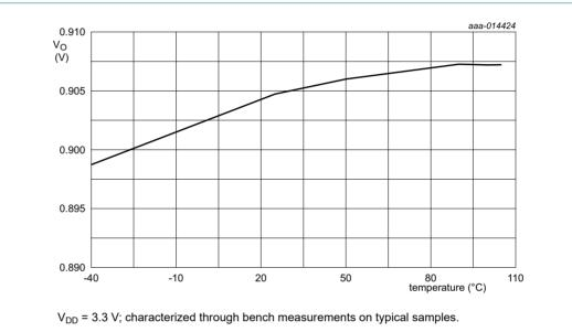
Fig 33. Typical internal voltage reference output voltage
