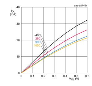
Conditions: V<sub>DD</sub> = 1.8 V; on pins PIO0\_10 and PIO0\_11.
