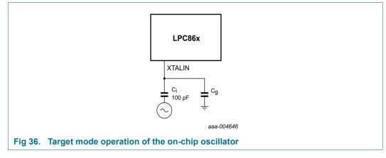
In target mode the input clock signal should be coupled with a capacitor of 100 pF (Figure 36), with an amplitude between 200 mV (RMS) and 1000 mV (RMS). This corresponds to a square wave signal with a signal swing of between 280 mV and 1.4 V. The XTALOUT pin in this configuration can be left unconnected.
