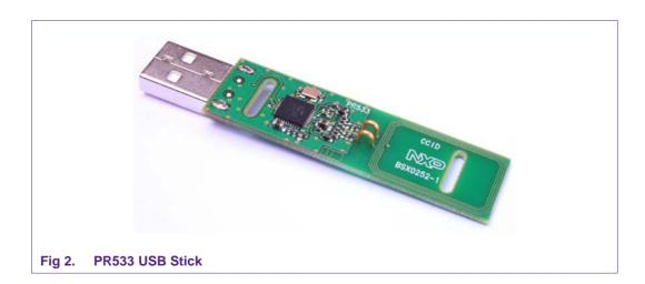
This evaluation board shows the simplest and smallest implementation of PR533 as USB reader. It is described in application note AN11064
