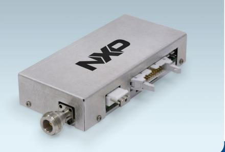
Complete reference design providing RF and real-time control for use in smart defrost applications
