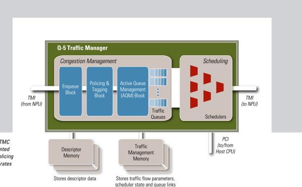
Flexible, look-aside TMC provides unprecedented traffic monitoring, policing and shaping at data rates up to 5Gbps
