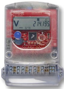
Electronic Tamper Detection Smart Meter Reference Design Using MMA8491Q Xtrinsic Tilt Threshold Sensor
