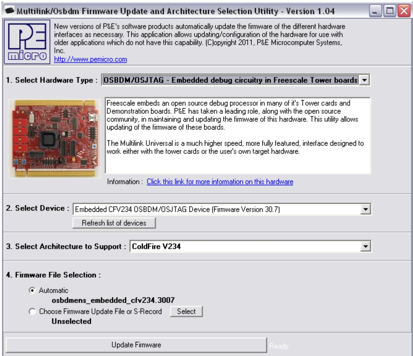
Click on “Update Firmware” to update the firmware. It will prompt you to disconnect the USB cord from your computer, and then short the JM60 boot loader jumper header for your particular board. It is the jumper labelled **BTLD** on the silk screen. For example, on the TWR-MCF52259 it is J20. On the TWR-MCF51CN it is J16. On the MCF52259DEMO it is J5. Then re-connect the board to your computer.
