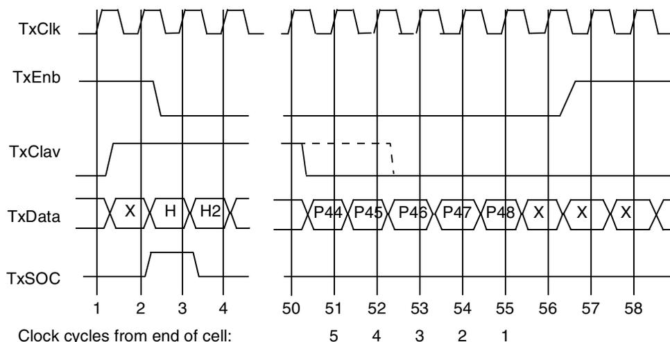
Figure 3. Transmit Timing for Cell-Level Handshake
