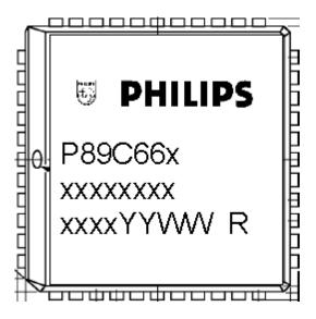
The last letter in the third line (field 'R') will identify the device revision. This Errata Sheet covers the following revisions of the P89C66x:
