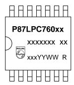
The last letter in the third line (field 'R') will identify the device revision. This Errata Sheet covers the following revisions of the P87LPC760:
