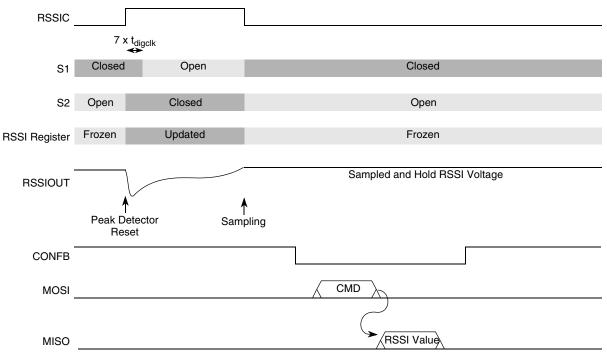
Figure 16. RSSI Operation in Sample Mode
