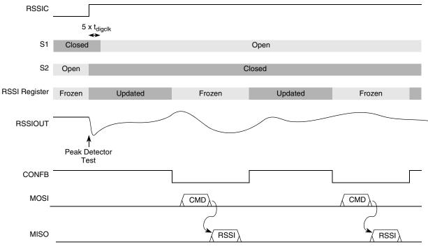
Figure 17. RSSI Operation in Continuous Mode
