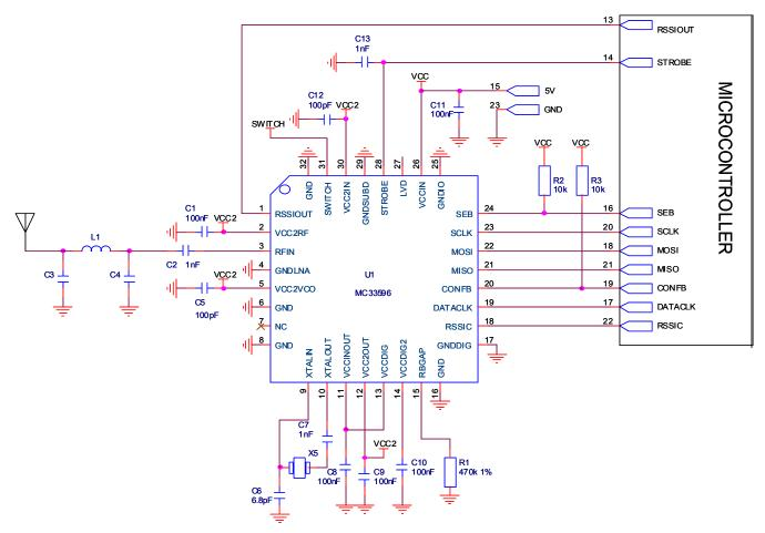
Figure 46. MC33596 Application Schematic in Strobe Mode (5 V)
