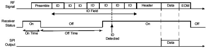
Figure 10. Complete Transmission with ID Detection
