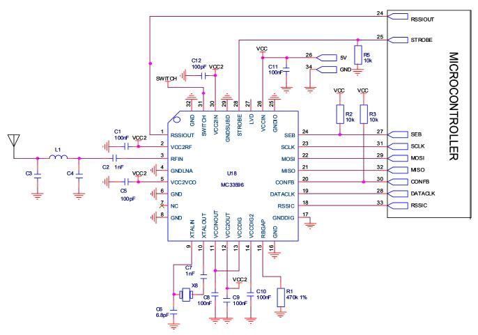
Figure 45. MC33596 Application Schematic (5 V)
