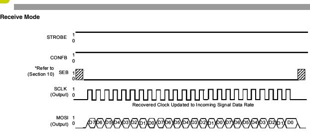
Figure 5. Typical Transfer in Receive mode with Data Manager
