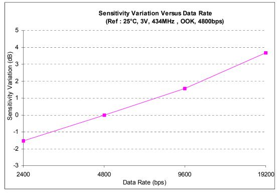
Figure 38. OOK Sensitivity Variation Versus Data Rate
