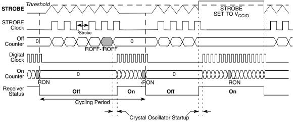
Figure 14. Receiver On/Off Sequence
