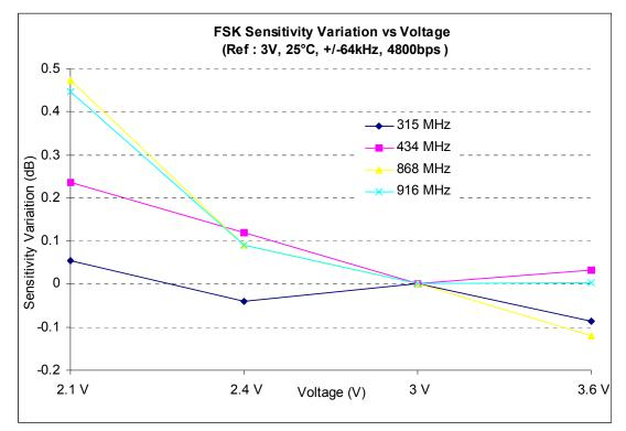
Figure 37. FSK Sensitivity Variation Versus Voltage
