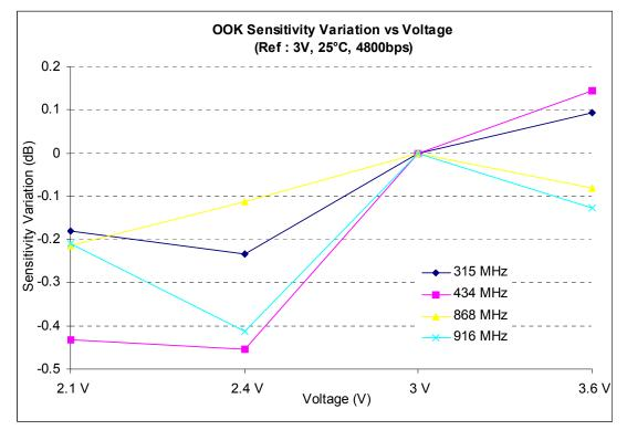
Figure 35. OOK Sensitivity Variation Versus Voltage
