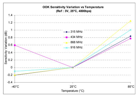
Figure 34. OOK Sensitivity Variation Versus Temperature
