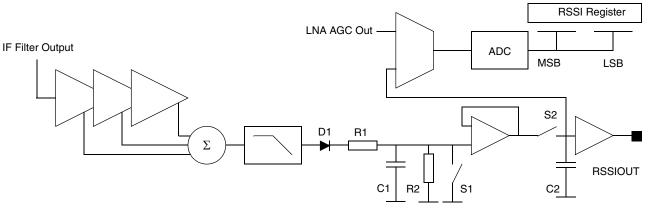
Figure 15. RSSI Simplified Block Diagram
