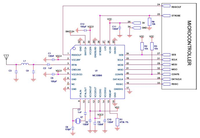
Figure 43. MC33596 Application Schematic (3 V)
