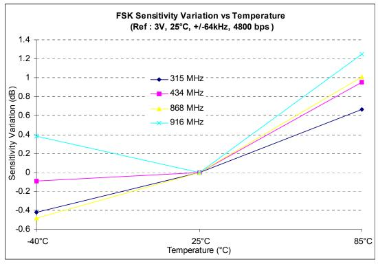
Figure 36. FSK Sensitivity Variation Versus Temperature
