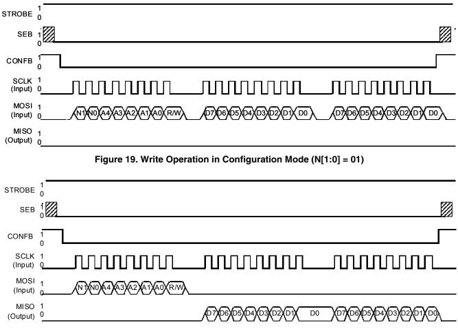
Figure 20. Read Operation in Configuration Mode (N[1:0] = 01)
