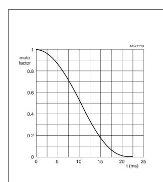
Fig.8 Mute as a function of raised cosine roll-off, displayed assuming 44.1 kHz.
