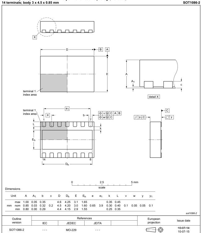
HVSON14: plastic, thermal enhanced very thin small outline package; no leads; 14 terminals; body 3 x 4.5 x 0.85 mm
