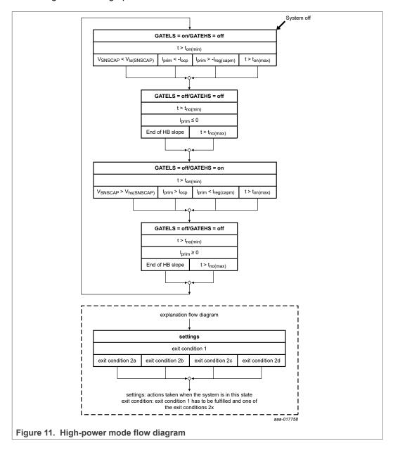
Initially, GATELS is on and GATEHS is off. The external bootstrap buffer capacitor ( $C_{SUPHS}$ ) is charged via the GATELS pin and an external diode. The system remains in this state for at least the minimum on-time ( $t_{on(min)}$ ) of GATELS. Before entering the next state, one of the following conditions must be fulfilled:
