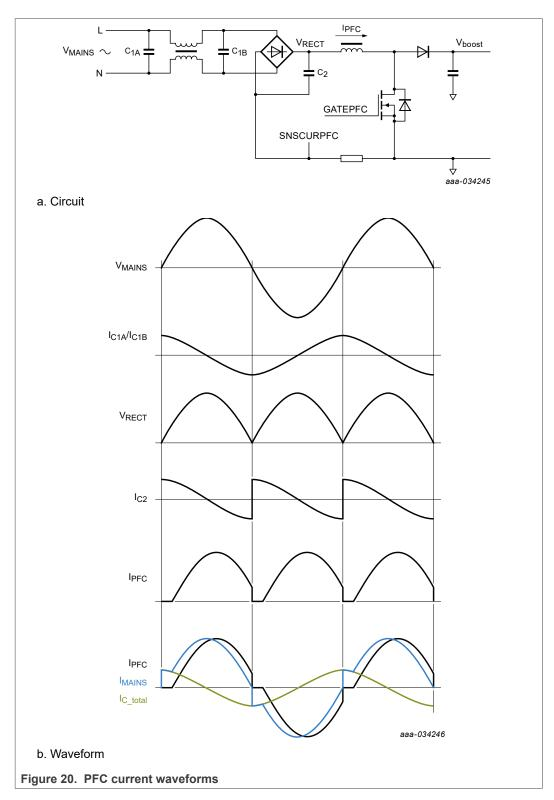
As the mains input current ( $I_{MAINS}$ ) is the sum of the current through the filter capacitances ( $I_{C\_total}$ ) and the PFC current ( $I_{PFC}$ ), it approaches a sine waveform.
