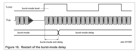
When the LLC is switching for a time that exceeds the burst-mode exit delay time and the output load exceeds the burst-mode level, the system leaves the burst mode. The burst-mode delay function is activated again. The burst-mode exit delay time can be set with a parameter.
