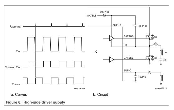
The external bootstrap buffer capacitor  $C_{SUPHS}$  supplies the high-side driver. The bootstrap capacitor is connected to the low-side driver supply, the GATELS pin, and the half-bridge node (HB) via an external diode ( $D_{SUPHS}$ ). When GATELS is active high and the HB node is pulled low,  $C_{SUPHS}$  is charged.
