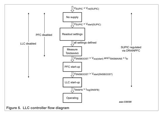
When the SUPIC voltage drops to below  $V_{\text{rst}(\text{SUPIC})}$ , the TEA2017AAT restarts.
