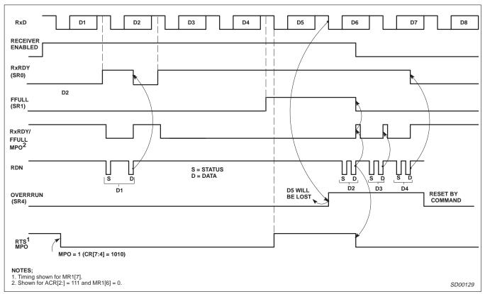
Figure 11. Receiver Timing
