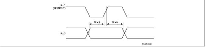
Figure 9. Receive Timing
