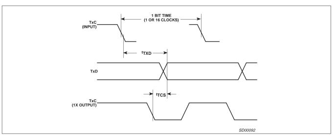
Figure 8. Transmit Timing
