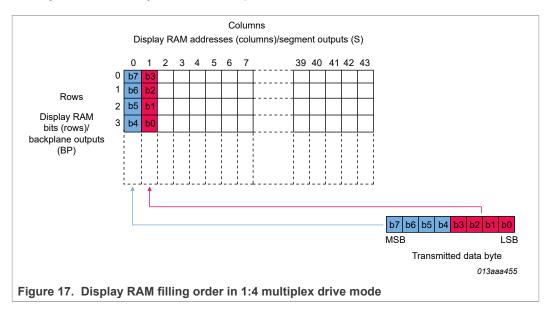
Depending on the start address of the data pointer, there is the possibility for a boundary condition. This occurs when more data bits are sent than fit into the remaining RAM. The additional data bits are discarded. See Figure 18.
