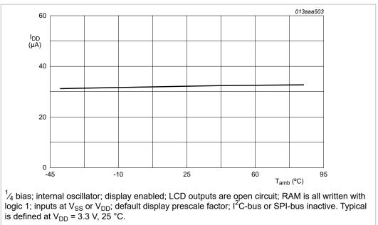
Figure 31. Typical I<sub>DD</sub> with respect to temperature
