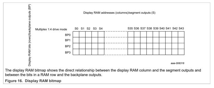
Logic 1 in the RAM bit map indicates the on-state ( $V_{on(RMS)}$ ) of the corresponding LCD element; similarly, logic 0 indicates the off-state ( $V_{off(RMS)}$ ). For more information on  $V_{on(RMS)}$  and  $V_{off(RMS)}$ , see Section 7.4.
