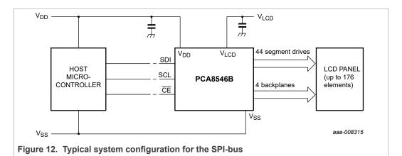
The host microcontroller maintains the two line  $I^2C$ -bus or a three line SPI-bus communication channel with the PCA8546. The appropriate biasing voltages for the multiplexed LCD waveforms are generated internally. The only other connections required to complete the system are the power supplies (V<sub>DD</sub>, V<sub>SS</sub>, V<sub>LCD</sub>) and the LCD panel selected for the application.
