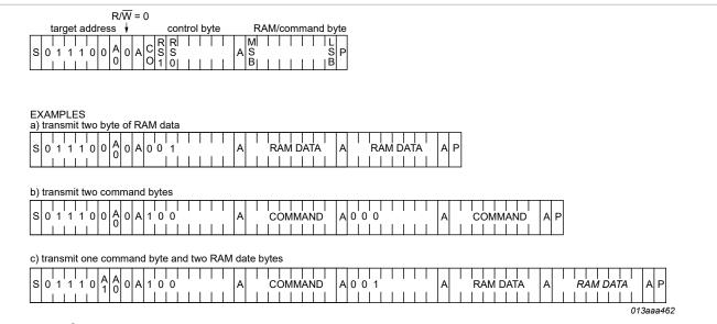
Figure 24. I<sup>2</sup>C-bus protocol write mode
