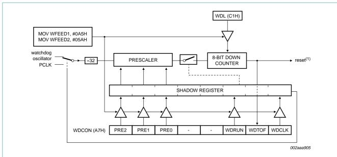
(1) Watchdog reset can also be caused by an invalid feed sequence, or by writing to WDCON not immediately followed by a feed sequence.
