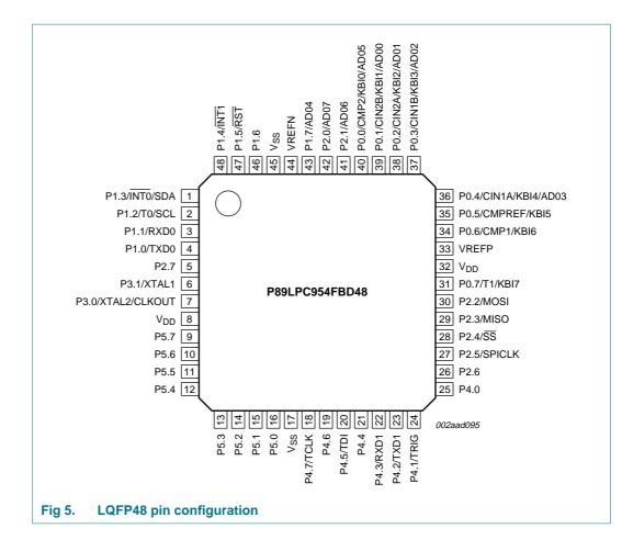
8-bit microcontroller with 10-bit ADC
