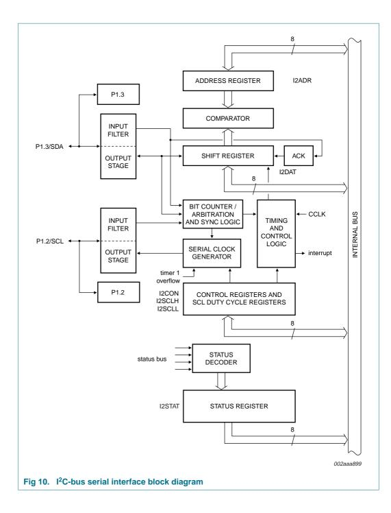
8-bit microcontroller with 10-bit ADC
