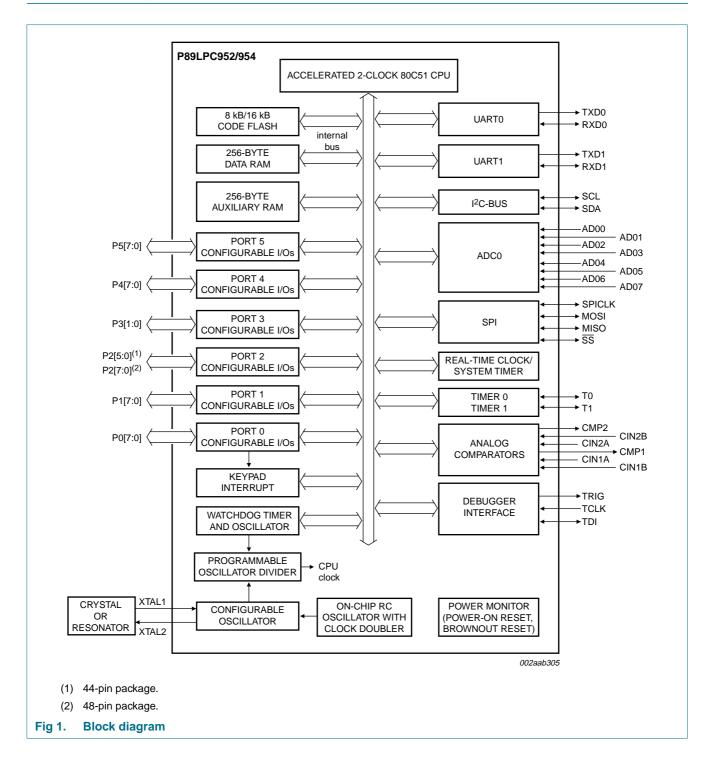
8-bit microcontroller with 10-bit ADC
