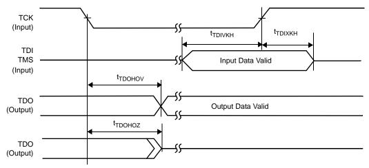
Figure 31. Test Access Port Timing
