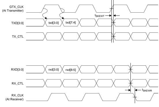
Figure 25. RGMII AC Timing and Multiplexing
