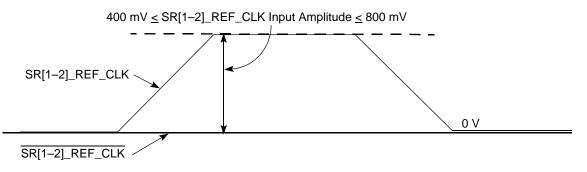
Figure 9. Single-Ended Reference Clock Input DC Requirements
