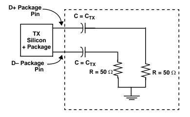
Figure 19. SGMII AC Test/Measurement Load
