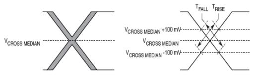
Figure 17. Single-Ended Measurement Points for Rise and Fall Time Matching
