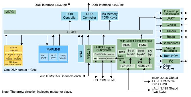
Figure 1. MSC8151 Block Diagram
