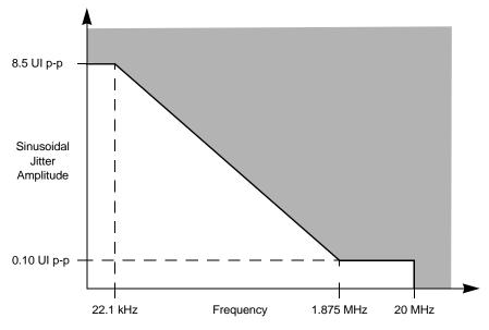
Figure 18. Single Frequency Sinusoidal Jitter Limits
