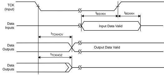
Figure 30. Boundary Scan (JTAG) Timing
