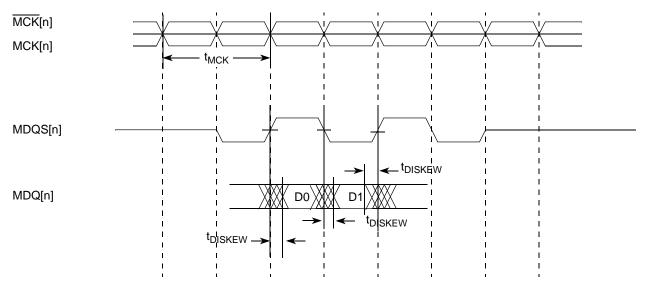
Figure 11. DDR2 and DDR3 SDRAM Interface Input Timing Diagram
