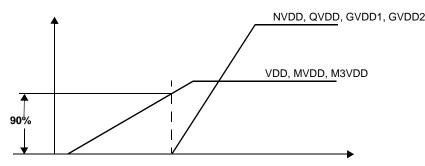
Figure 34. Supply Ramp-Up Sequence
