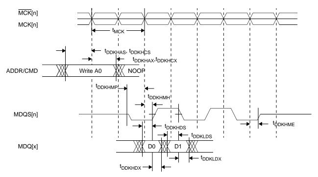
Figure 13. DDR SDRAM Output Timing
