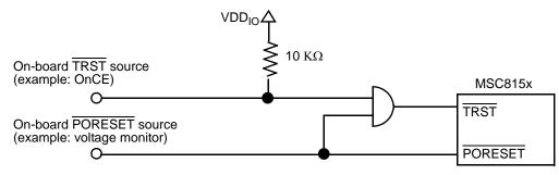
Figure 36. Reset Connection in Debugger Application
