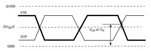
Figure 15. DDR2 and DDR3 SDRAM Differential Timing Specifications
