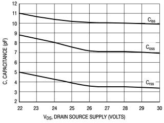
Figure 10. Capacitance versus Drain Source Voltage
