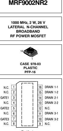
(Top View) Note: Exposèd backside flag is source terminal for transistors.
