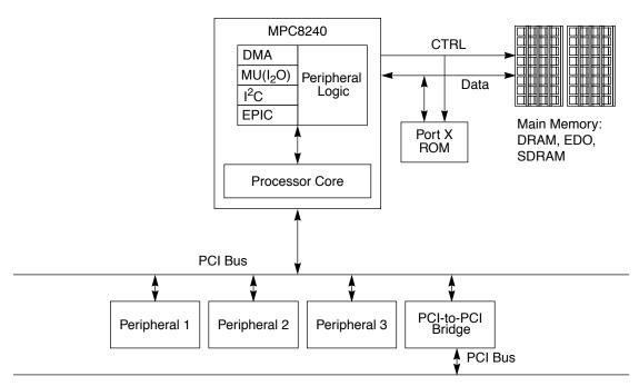
Figure 1-2. System Using an Integrated MPC8240 as a Host Processor
