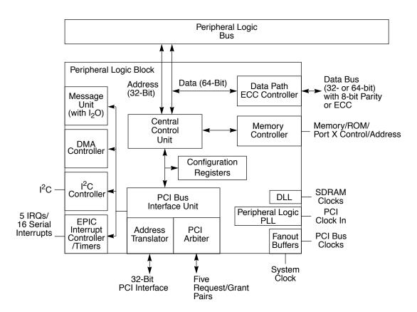
Figure 1-6. MPC8240 Peripheral Logic Block Diagram
