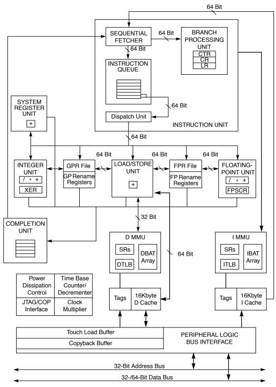
Figure 1-5. MPC8240 Integrated Processor Core Block Diagram
