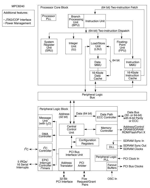
Figure 1-1. MPC8240 Integrated Processor Functional Block Diagram
