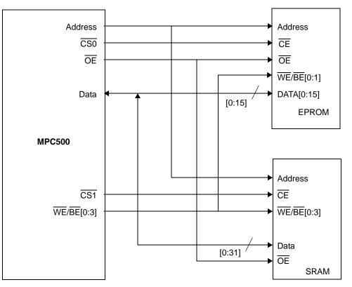
Figure 10-3. MPC565 Simple System Configuration
