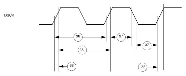
Figure F-28. Debug Port Clock Input Timing
