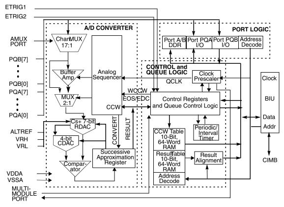
Figure 13-2. QADC64E Block Diagram
