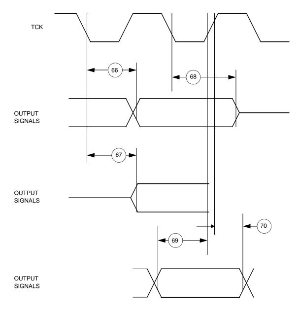
Figure F-39. Boundary Scan (JTAG) Timing Diagram
