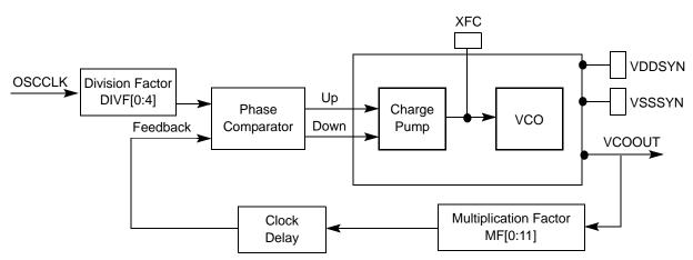
Figure 8-3. System PLL Block Diagram
