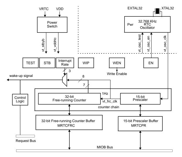
Figure 17-47. MRTCSM Block Diagram
