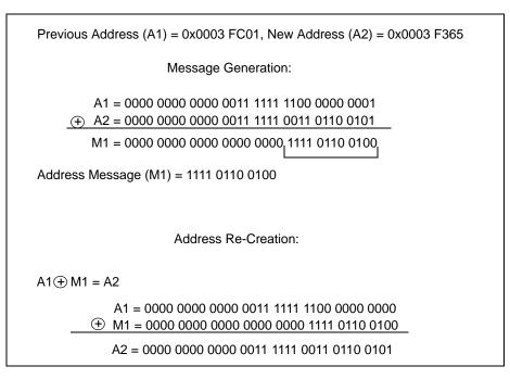
Figure 23-32. Relative Address Generation and Re-Creation
