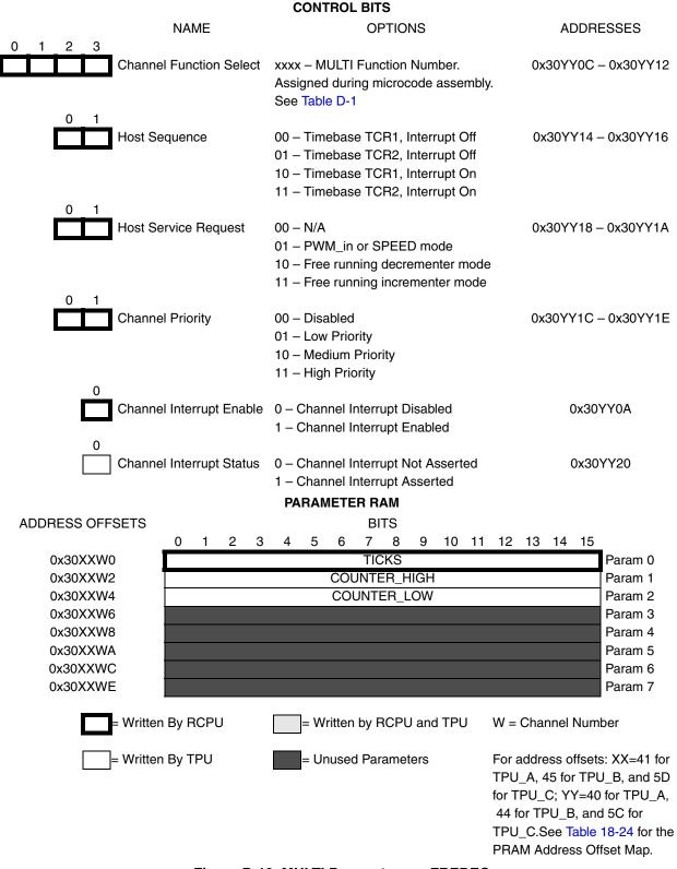
Figure D-19. MULTI Parameters — FREDEC
