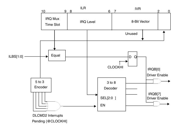
Figure 15-39. DLCMD2 Interrupt Vector Generation (IRQ\_PLUG = 1)
