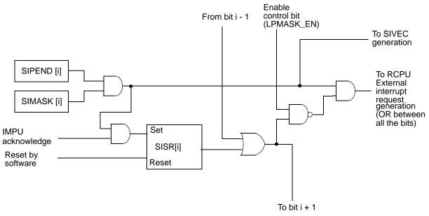
Figure 6-4. Lower Priority Request Masking—One Bit Diagram
