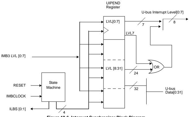
Figure 12-6. Interrupt Synchronizer Block Diagram
