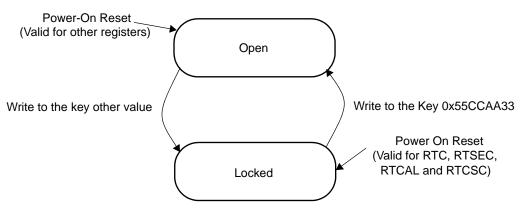
Figure 8-12. Keep-Alive Register Key State Diagram
