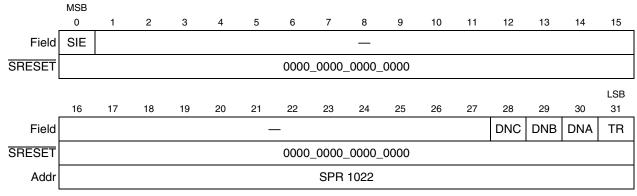
Figure 3-18. Floating-Point Exception Cause Register (FPECR)
