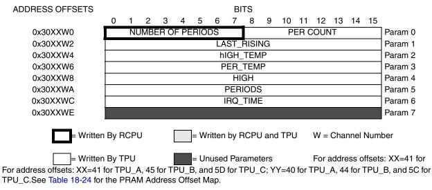
Figure D-21. MULTI Parameters — PWM\_IN
