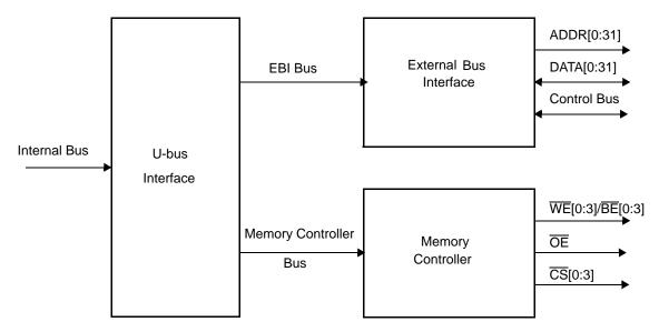
Figure 10-1. Memory Controller Function within the USIU
