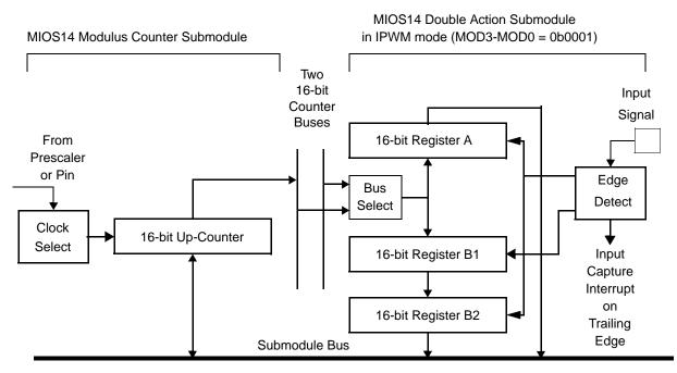
Figure 17-43. MIOS14 Example: Double Capture Pulse Width Measurement
