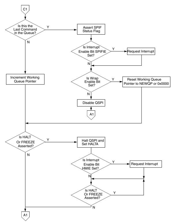
Figure 14-21. Flowchart of QSPI Master Operation (Part 3)
