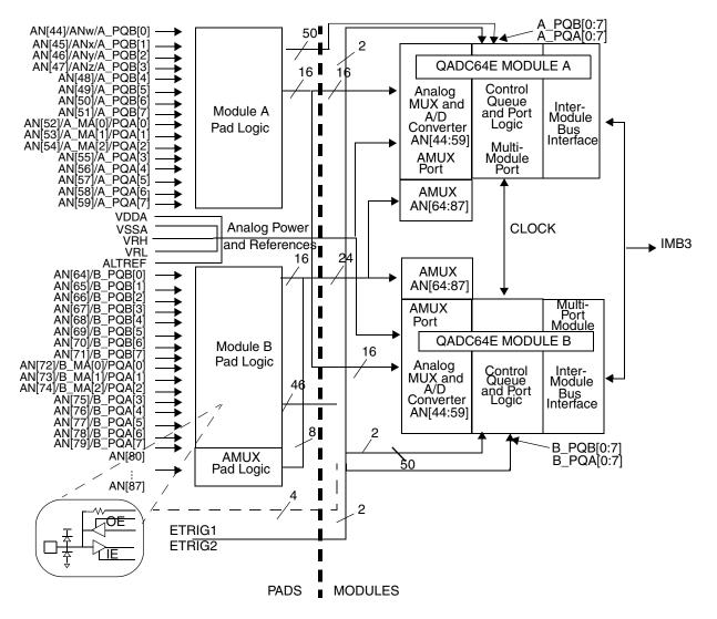
Figure 13-1. Dual QADC64Es on the MPC565
