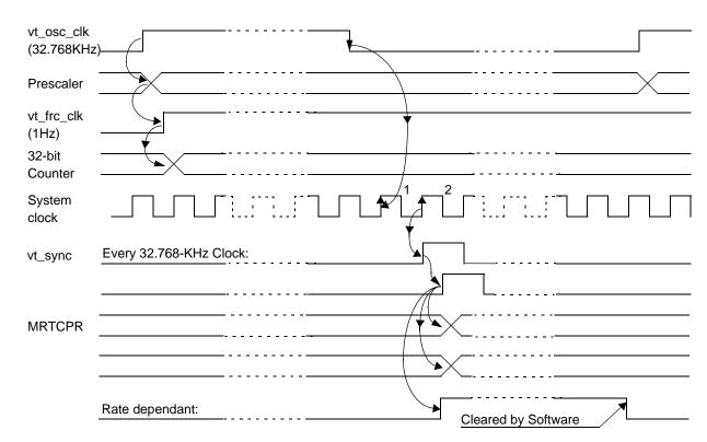
Figure 17-50. 15-Bit Prescaler and 32-Bit Free-Running Counter Buffer Updates
