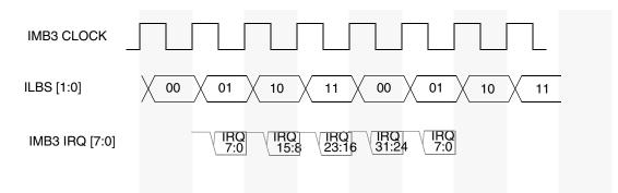
Figure 13-7. Interrupt Levels on IRQ with ILBS
