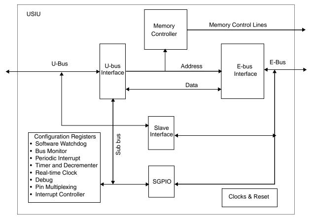
Figure 5-1. USIU Block Diagram
