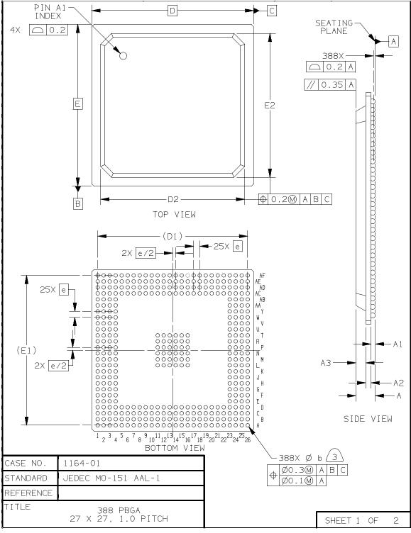
Figure F-62. MPC565 Package Footprint (1 of 2)
