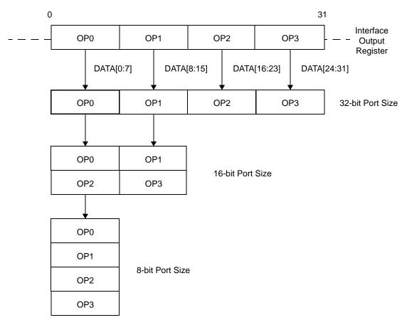
Figure 9-23 illustrates the device connections on the data bus.
