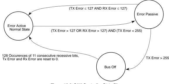
Figure 16-6. CAN Controller State Diagram
