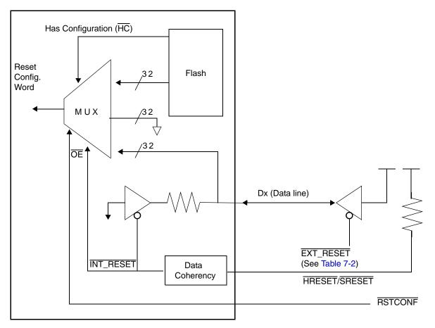
Figure 7-2. Reset Configuration Basic Scheme
