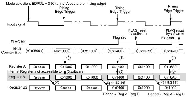
Figure 17-17. Input Period Measurement Example
