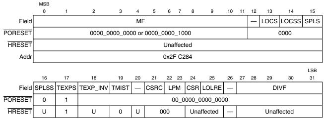
Figure 8-16. PLL, Low-Power, and Reset-Control Register (PLPRCR)
