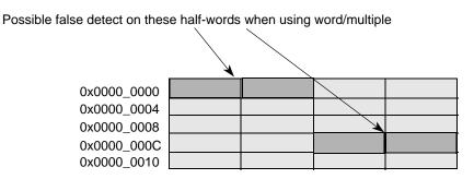
Figure 22-2. Partially Supported Watchpoint/Breakpoint Example
