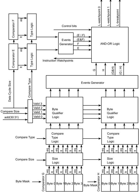
Figure 22-4. Load/Store Support General Structure
