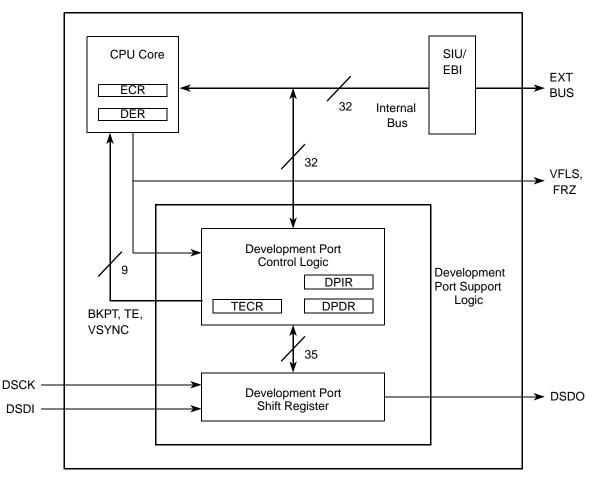
Figure 22-5. Functional Diagram of MPC565 Debug Mode Support
