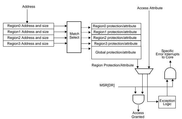
Figure 11-2. DMPU Basic Functional Diagram
