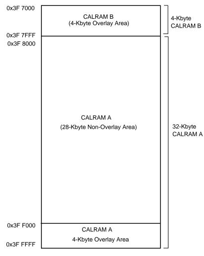
Figure 21-6. CALRAM B and CALRAM A Address Map (When CLPS = 0)
