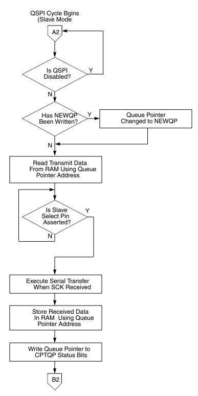
Figure 14-22. Flowchart of QSPI Slave Operation (Part 1)
