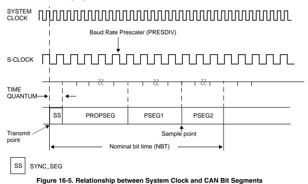
A bit is divided into four separate non-overlapping time segments called SYNC\_SEG, PROPSEG, PSEG1, and PSEG2. These are illustrated in Figure 16-5. The period of the nominal bit time (NBT) is the sum of the segment durations:
