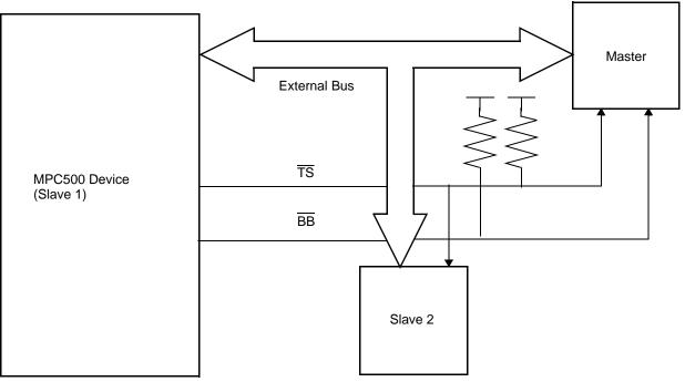
Figure 9-25. Master Signals Basic Connection
