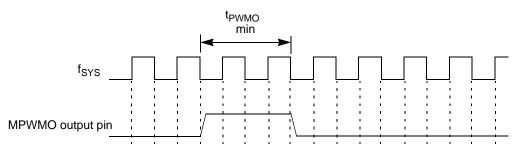
Figure F-46. MPWMSM Minimum Output Pulse Example Timing Diagram
