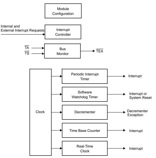
Figure 6-1. System Configuration and Protection Logic
