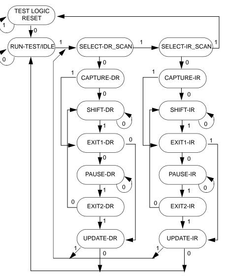
Figure 24-3. TAP Controller State Machine
