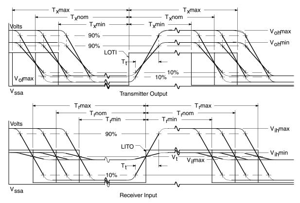
J1850 bus transmitter output and input signal waveforms are shown in Figure 15-3.
