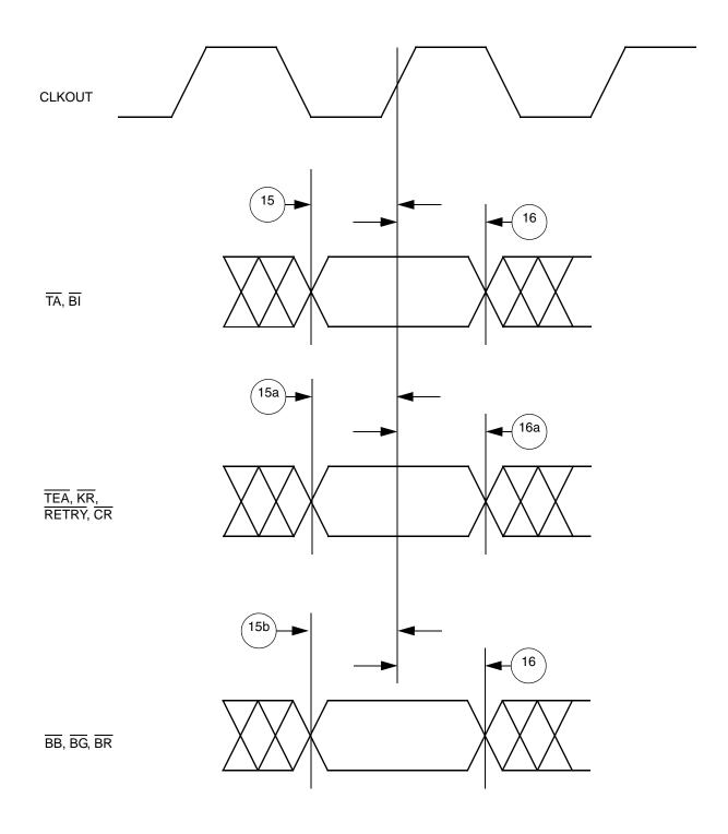
Figure F-14. Synchronous Input Signals Timing
