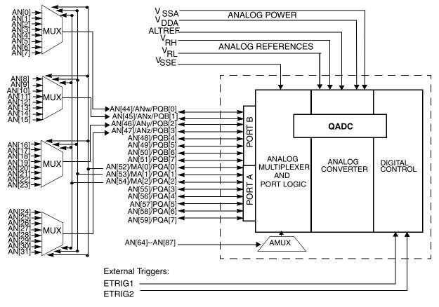
Figure 13-4. Example of External Multiplexing
