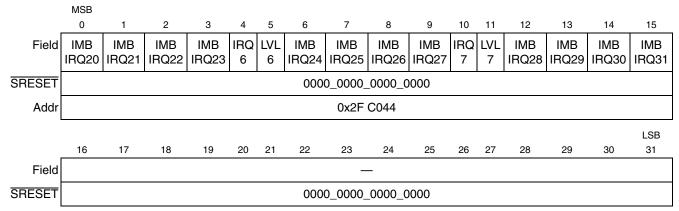
Figure 6-17. SIU Interrupt Pending Register 3 (SIPEND3)
