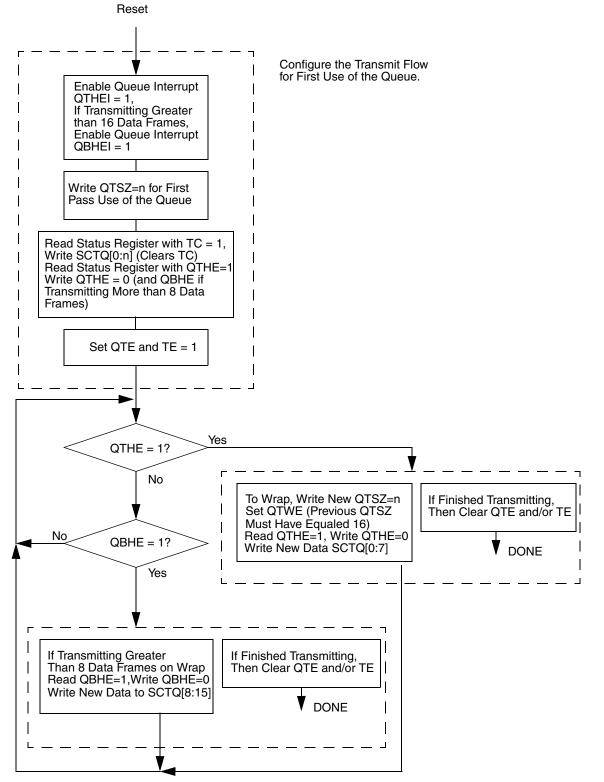
Figure 14-35. QSCI1 Queue Transmit Software Flow
