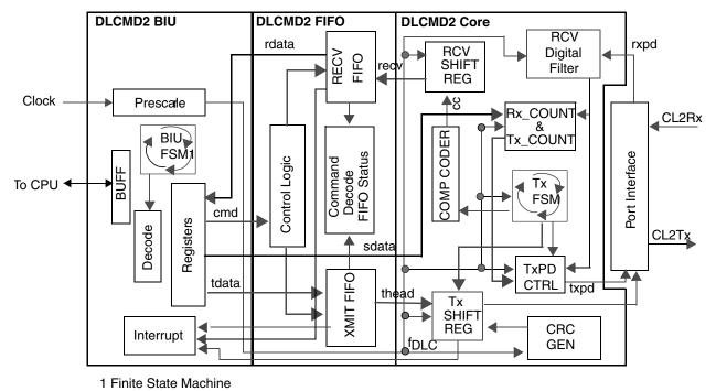
Figure 15-1. DLCMD2 Block Diagram
