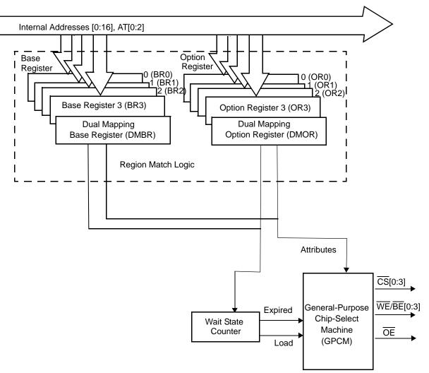
Figure 10-2. Memory Controller Block Diagram
