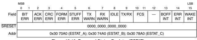
Figure 16-19. Error and Status Register (ESTAT)
