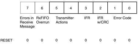
Figure 15-31. Completion Code Byte Bit Definitions
