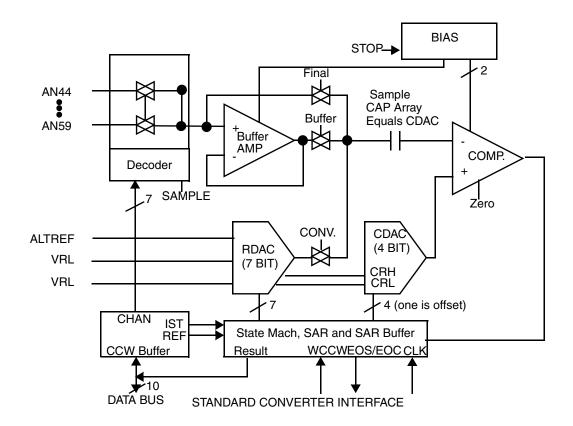
Figure 13-21. QADC64E Analog Subsystem Block Diagram
