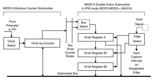
Figure 17-44. MIOS14 Example: Double Capture Period Measurement
