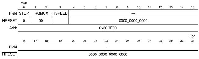
Figure 12-7. UIMB Module Configuration Register (UMCR)
