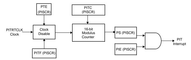
Figure 6-8. PIT Block Diagram
