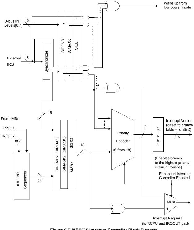
Figure 6-5. MPC565 Interrupt Controller Block Diagram
