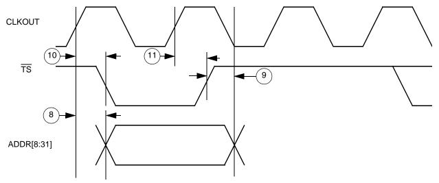
Figure F-20. Address Show Cycle Bus Timing
