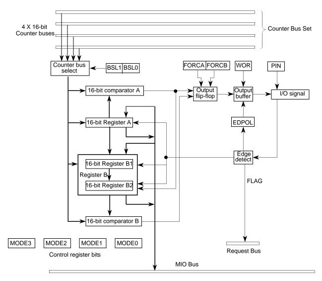
Figure 17-15. MDASM Block Diagram
