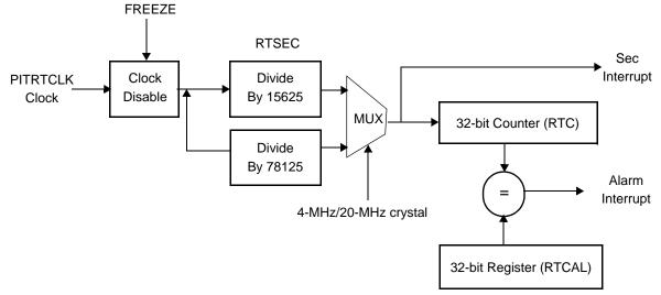
Figure 6-7. RTC Block Diagram
