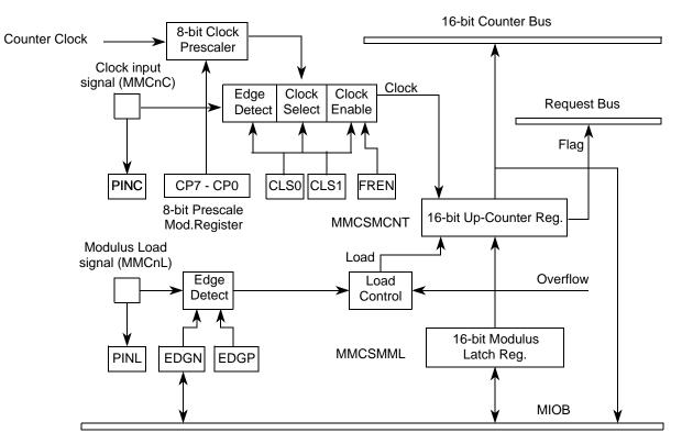
Figure 17-10. MMCSM Block Diagram
