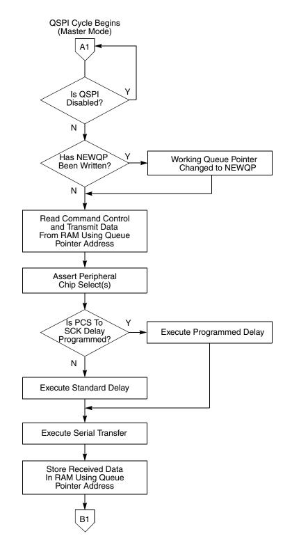
Figure 14-19. Flowchart of QSPI Master Operation (Part 1)
