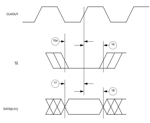
Figure F-15. Input Data Timing In Normal Case
