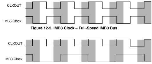
Figure 12-3. IMB3 Clock – Half-Speed IMB3 Bus
