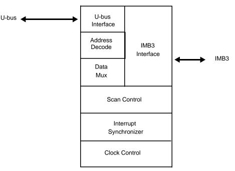
Figure 12-1. UIMB Interface Module Block Diagram
