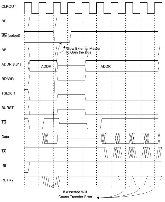
Figure 9-34. Retry on Burst Cycle
