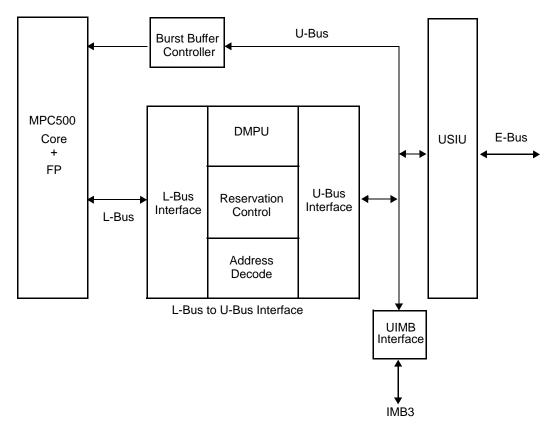
Figure 11-1. L2U Bus Interface Block Diagram
