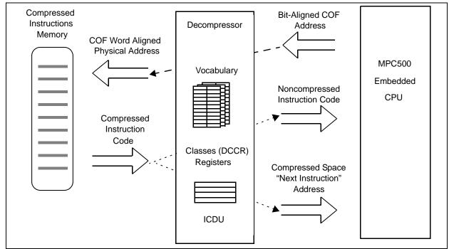
Figure A-12. Code Decompression Process
