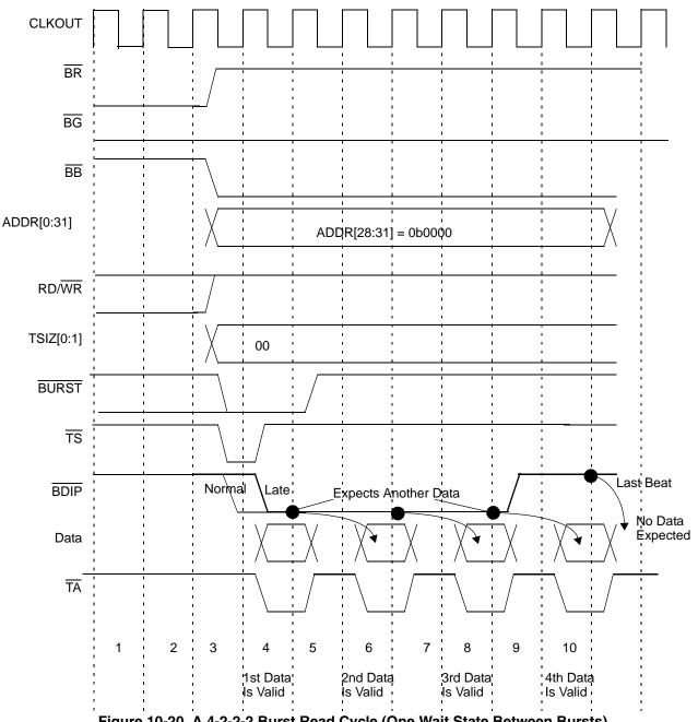
Figure 10-20. A 4-2-2-2 Burst Read Cycle (One Wait State Between Bursts)
