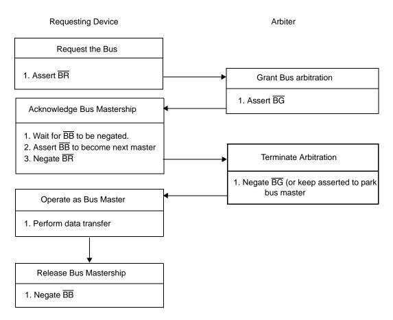
Figure 9-24. Bus Arbitration Flowchart
