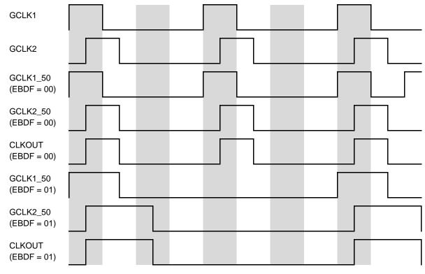
Figure 8-7. Clocks Timing For DFNH = 1 (or DFNL = 0)
