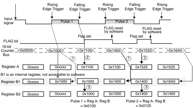
Mode selection; EDPOL = 1 (Channel A capture on falling edge, Channel B capture on rising edge)
