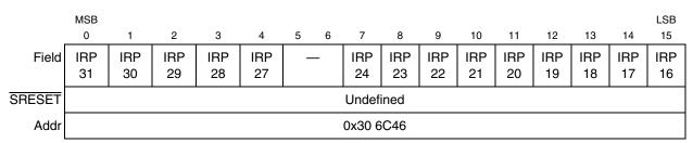
Figure 17-40. Interrupt Request Pending Register (MIOS14RPR1)
