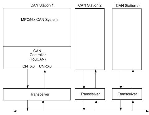
Figure 16-2. Typical CAN Network
