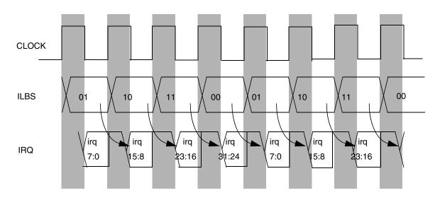
Figure 15-38. Interrupt Request Multiplex Timing
