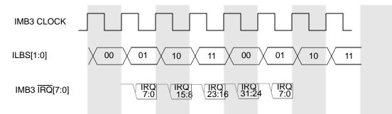
Figure 18-2. TPU3 Interrupt Levels
