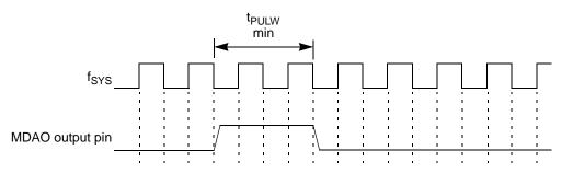
Figure F-58. MDASM Minimum Output Pulse Width Timing Diagram
