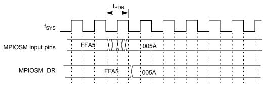
Figure F-61. MPIOSM Input Pin to MPIOSM\_DR (Data Register) Timing Diagram
