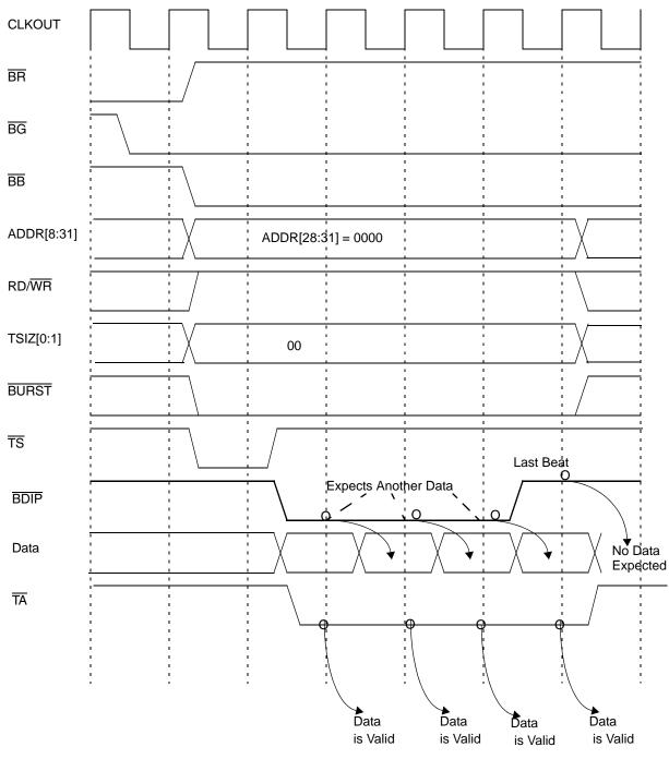
Figure 9-12. Basic Flow Diagram Of A Burst-Read Cycle
