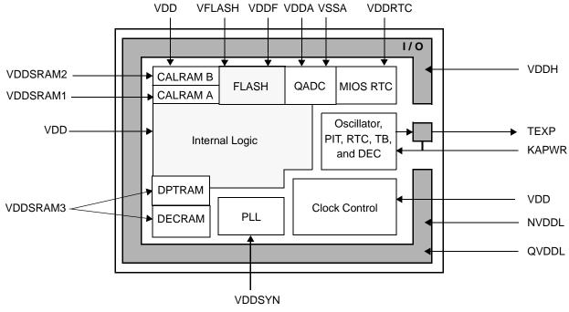
Figure 8-10. Basic Power Supply Configuration
