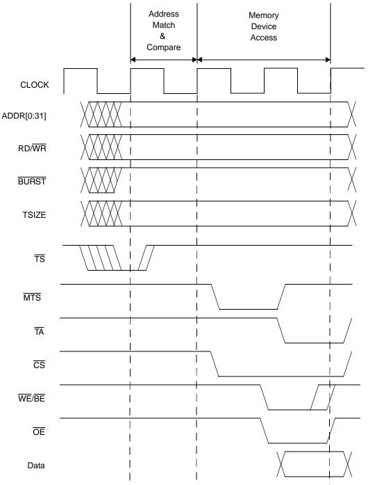
Figure 10-19. Synchronous External Master Basic Access (GPCM Controlled)
