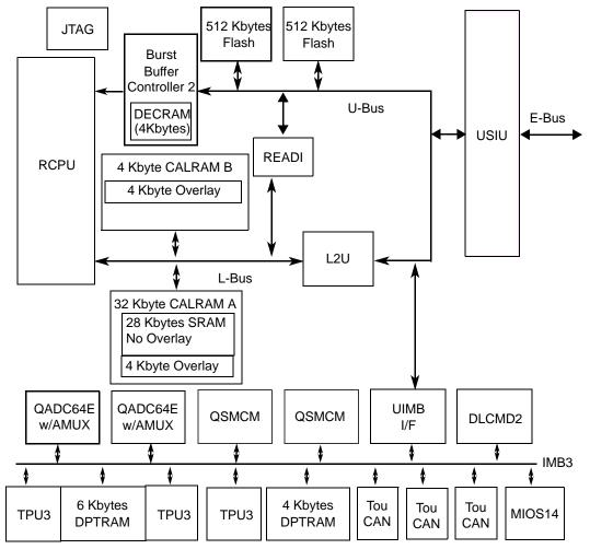
Figure 1-1. MPC565 Block Diagram
