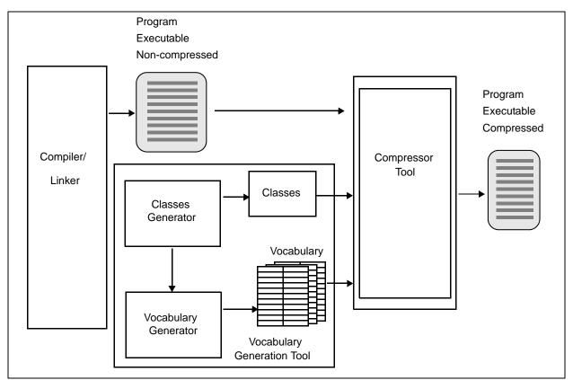
Figure A-11. Code Compression Process
