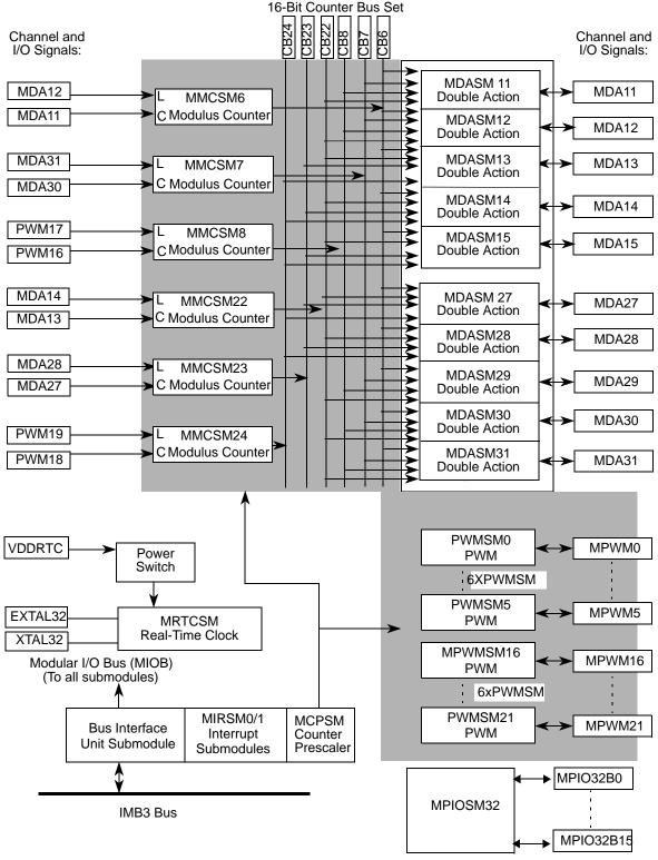
Figure 17-1. MPC565 MIOS14 Block Diagram
