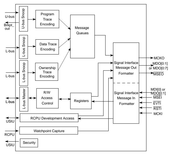
Figure 23-1. READI Functional Block Diagram
