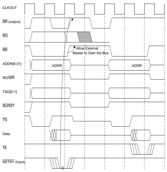
Figure 9-33. Retry Transfer Timing – External Arbiter
