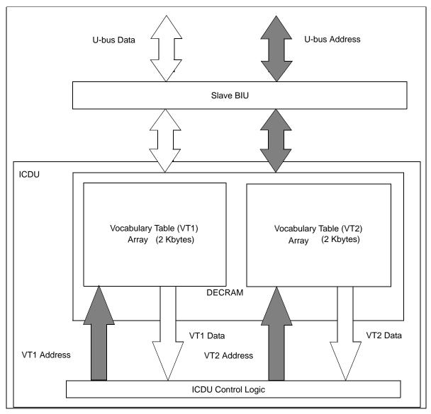
Figure 4-4. DECRAM Interfaces Block Diagram
