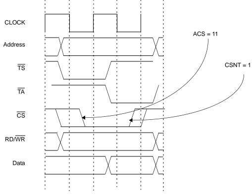
Figure 10-8. Peripheral Devices Basic Timing (ACS = 11, TRLX = 0)
