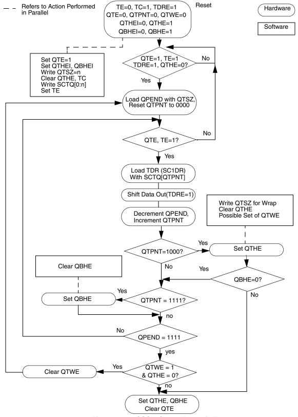
Figure 14-34. QSCI1 Queue Transmit Flow
