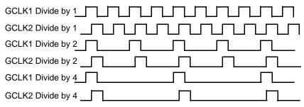
Figure 8-6. Divided System Clocks Timing Diagram
