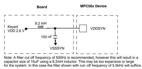
Figure C-7. LC Filter Example (Alternative)
