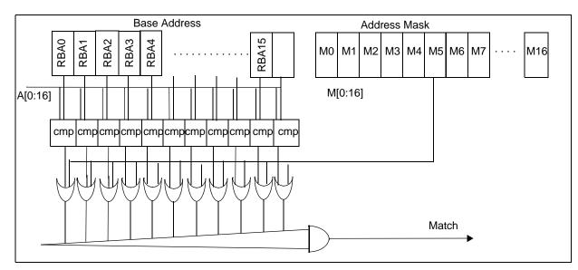
Figure 10-4. Bank Base Address and Match Structure
