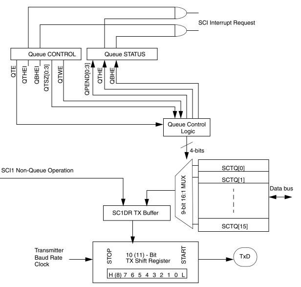
Figure 14-33. Queue Transmitter Block Enhancements
