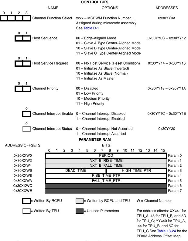
Figure D-14. MCPWM Parameters — Slave Ch A Non-Inverted Center-Aligned Mode
