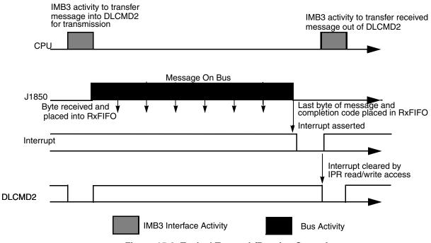
Figure 15-2. Typical Transmit/Receive Operation
