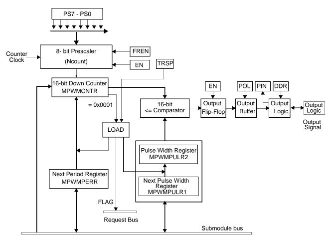
Figure 17-25. MPWMSM Block Diagram
