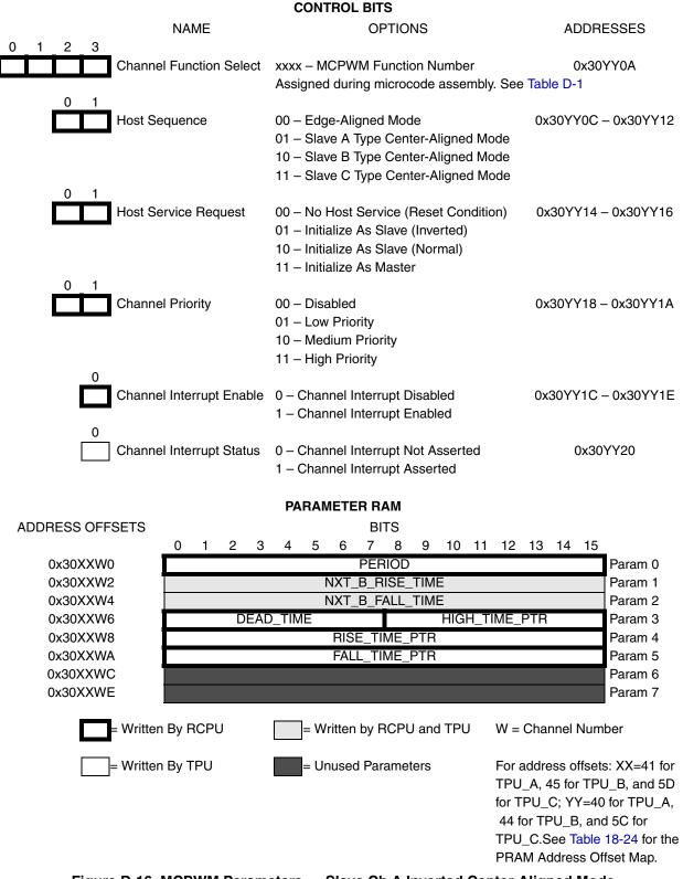
Figure D-16. MCPWM Parameters — Slave Ch A Inverted Center-Aligned Mode
