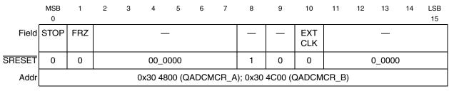
Figure 13-5. Module Configuration Register (QADCMCR)
