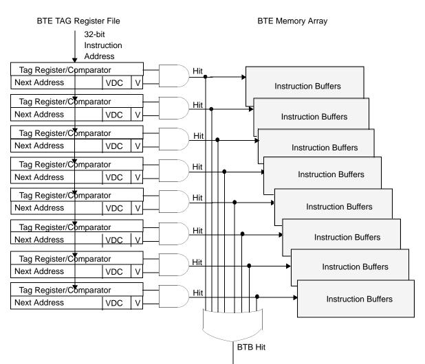
Figure 4-5. BTB Block Diagram
