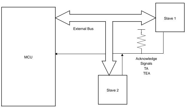
Figure 9-28. Termination Signals Protocol Basic Connection
