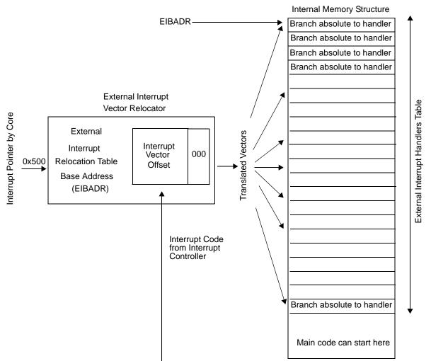
Figure 4-3. External Interrupt Vectors Splitting
