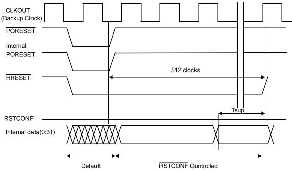
Figure 7-4. Reset Configuration Timing for "Short" PORESET Assertion, Limp Mode Enabled
