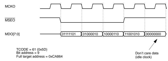
Figure 23-42. Indirect Branch Synchronization Message with Compressed Code
