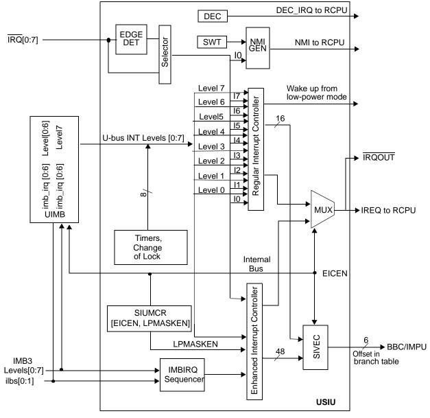
Figure 6-3. MPC565 Interrupt Structure
