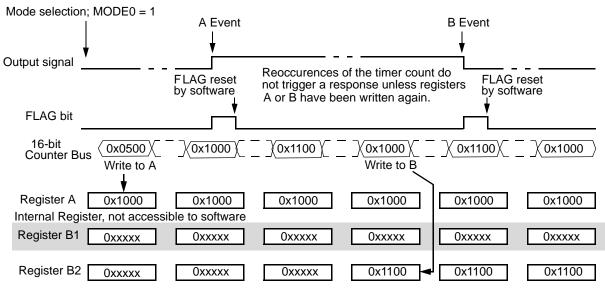
Figure 17-20. Single Shot Output Transition Example
