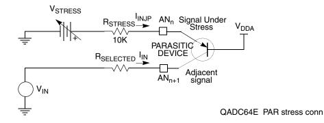
Figure 13-54. Input Signal Subjected to Positive Stress
