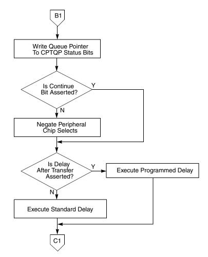
Figure 14-20. Flowchart of QSPI Master Operation (Part 2)
