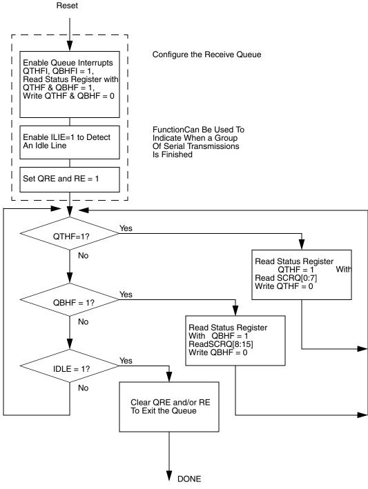
Figure 14-40. Queue Receive Software Flow
