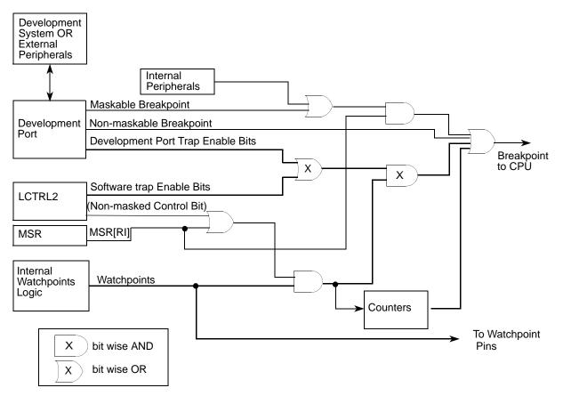
Figure 22-1. Watchpoint and Breakpoint Support in the CPU
