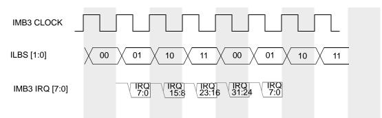
Figure 16-7. Interrupt Levels on IRQ with ILBS
