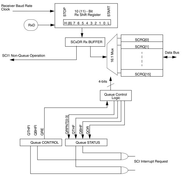
Figure 14-38. Queue Receiver Block Enhancements
