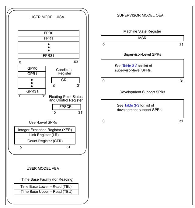
Figure 3-3. RCPU Programming Model
