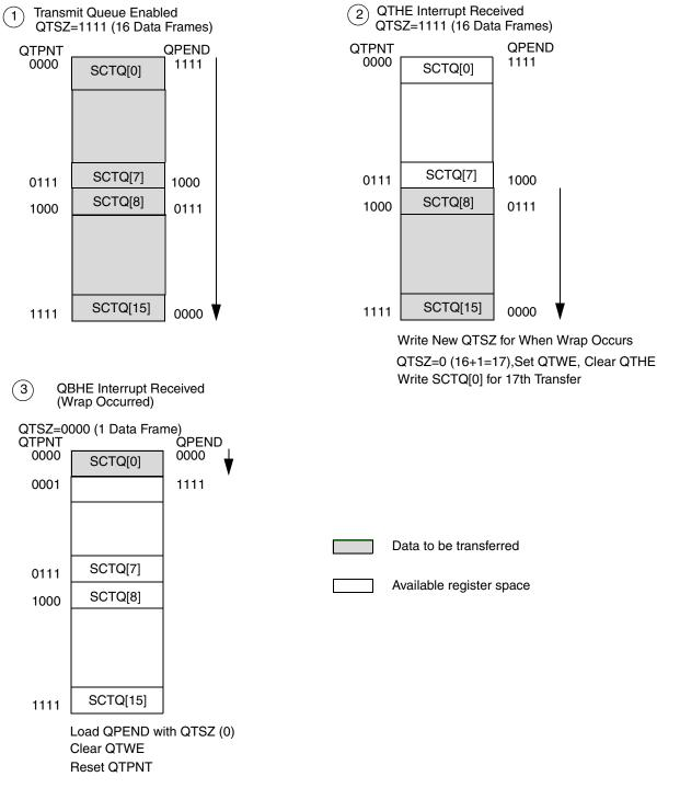
Figure 14-36. Queue Transmit Example for 17 Data Bytes
