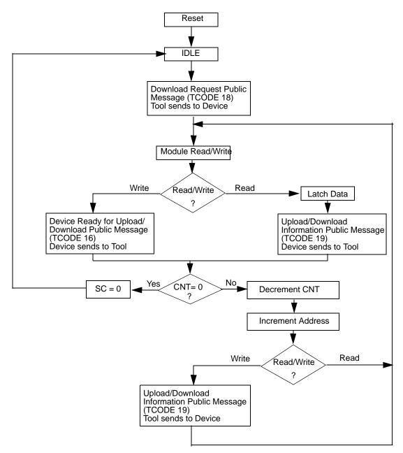
Figure 23-58. Read/Write Access Flow Diagram
