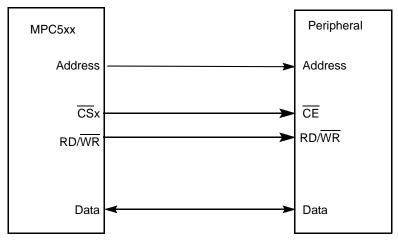
Figure 10-7. Peripheral Devices Interface
