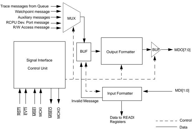
Figure 23-11. Functional Diagram of Signal Interface
