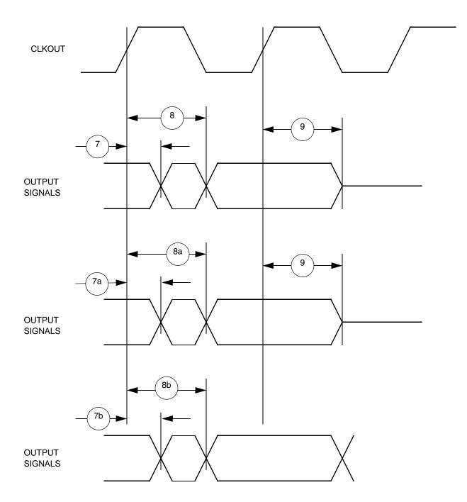
Figure F-11. Synchronous Output Signals Timing
