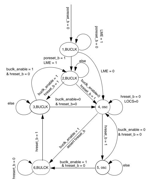
Figure 8-8. Clock Source Switching Flow Chart
