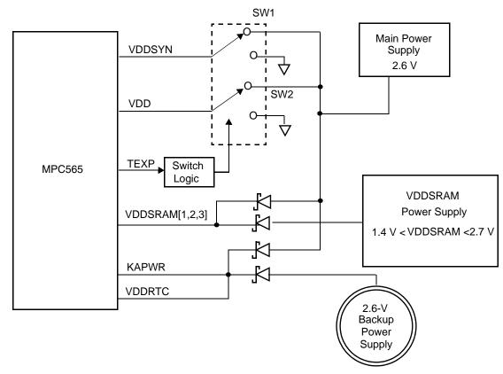
Figure 8-11. External Power Supply Scheme
