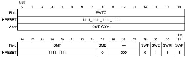
Figure 6-26. System Protection Control Register (SYPCR)
