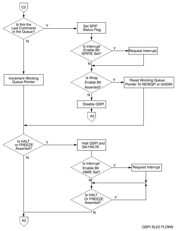
Figure 14-23. Flowchart of QSPI Slave Operation (Part 2)
