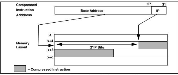
Figure A-2. Addressing Instructions with Compressed Address
