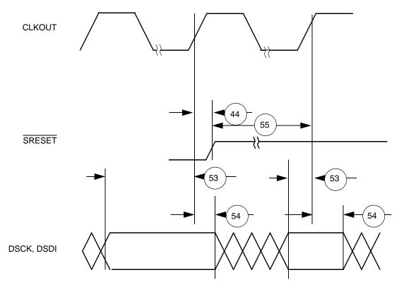
Figure F-36. Reset Timing – Debug Port Configuration
