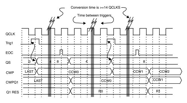
Figure 13-45. External Trigger Mode (Positive Edge) Timing With Pause
