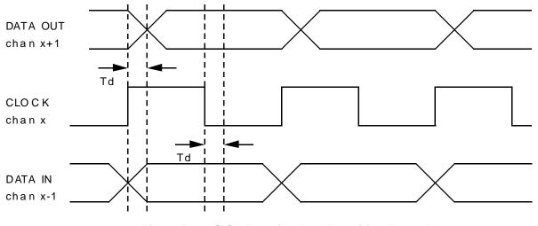
Figure D-33. SIOP Function Data Transition Example
