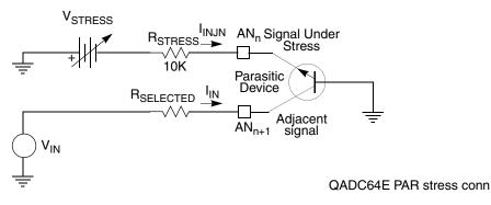
Figure 13-53. Input Signal Subjected to Negative Stress
