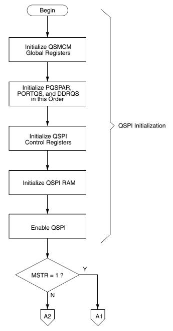
Figure 14-18. Flowchart of QSPI Initialization Operation
