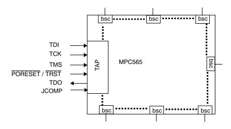
Figure 24-1. Pin Requirement on JTAG
