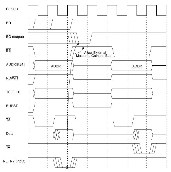
Figure 9-32. Retry Transfer Timing – Internal Arbiter
