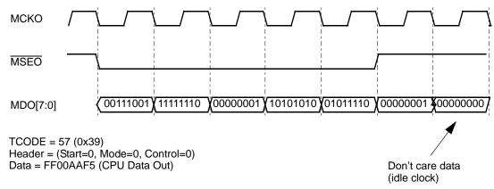
Figure 23-88. DSDO Data Message (CPU Data Out)
