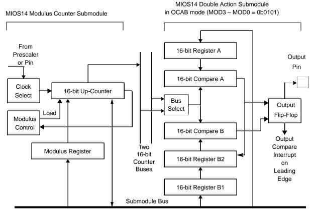
Figure 17-46. MIOS14 Example: Pulse Width Modulation Output
