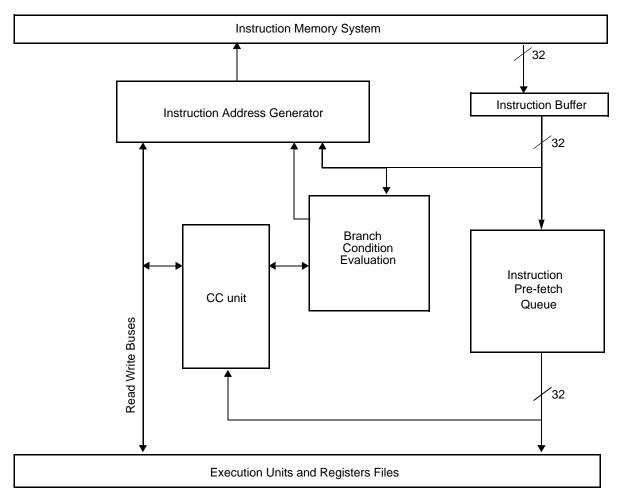
Figure 3-2. Sequencer Data Path
