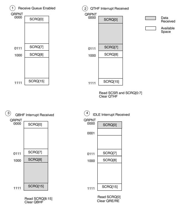
Figure 14-41. Queue Receive Example for 17 Data Bytes
