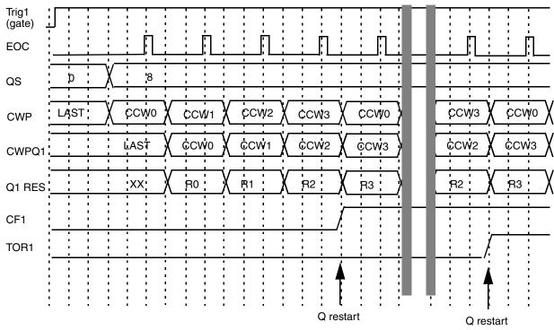
Figure 13-47. Gated Mode, Continuous Scan Timing
