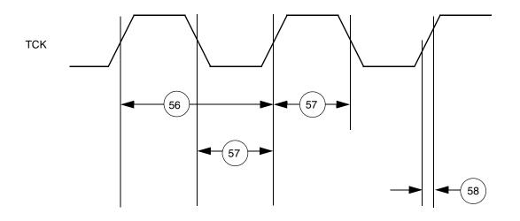
Figure F-37. JTAG Test Clock Input Timing
