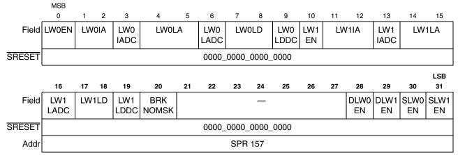
Figure 22-22. L-Bus Support Control Register 2 (LCTRL2)
