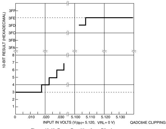
Figure 13-49. Errors Resulting from Clipping
