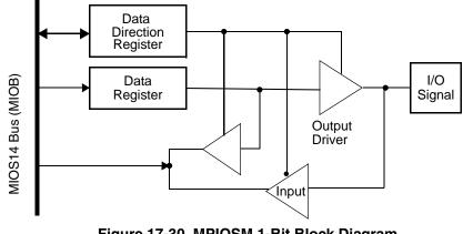
Figure 17-30. MPIOSM 1-Bit Block Diagram
