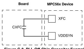
Figure C-8. PLL Off-Chip Capacitor Example
