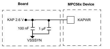
Figure C-5. Bypass Capacitors Example (Alternative)
