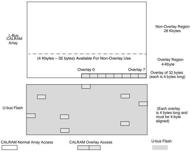
Figure 21-7. CALRAM Module Overlay Map of Flash (CLPS = 1)
