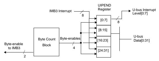
Figure 12-4. Interrupt Synchronizer Signal Flow
