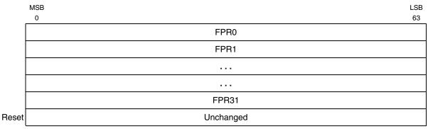
Figure 3-5. Floating-Point Registers (FPRs)
