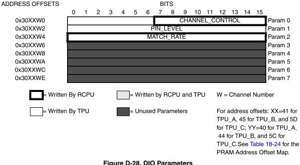
Figure D-28. DIO Parameters
