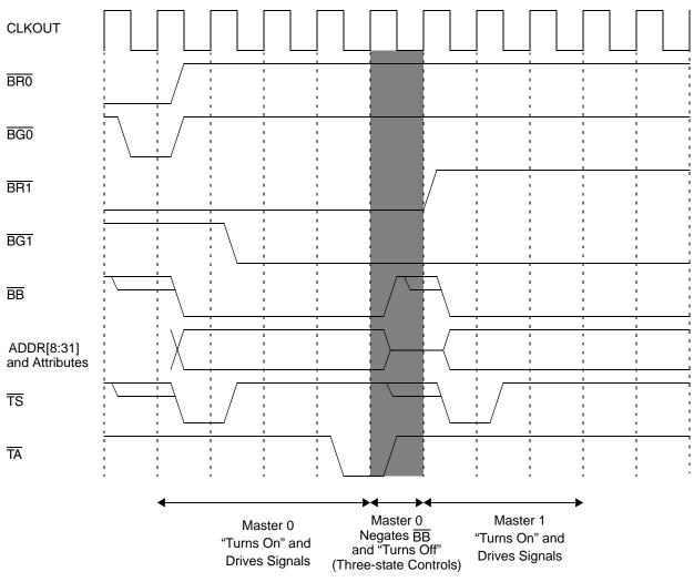
Figure 9-26. Bus Arbitration Timing Diagram
