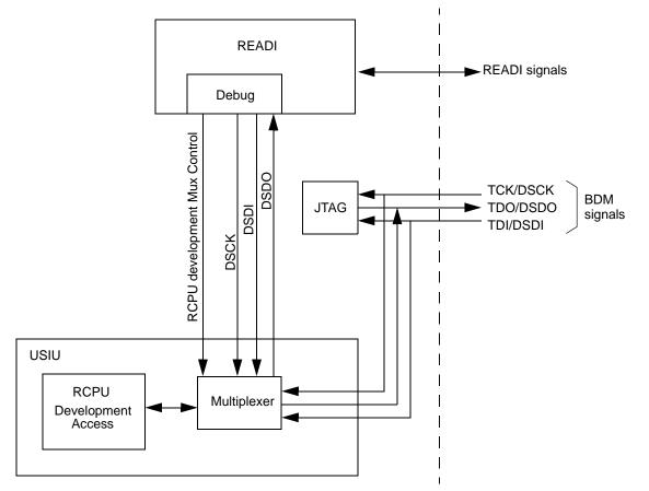
Figure 23-77. RCPU Development Access Multiplexing between READI and BDM Signals
