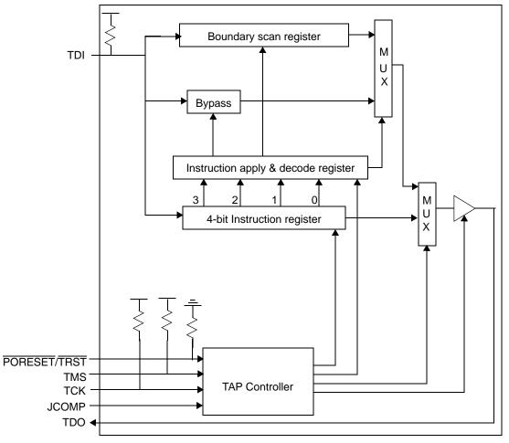
Figure 24-2. Test Logic Block Diagram
