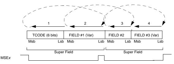
Figure 23-14. Transmission Sequence of Messages
