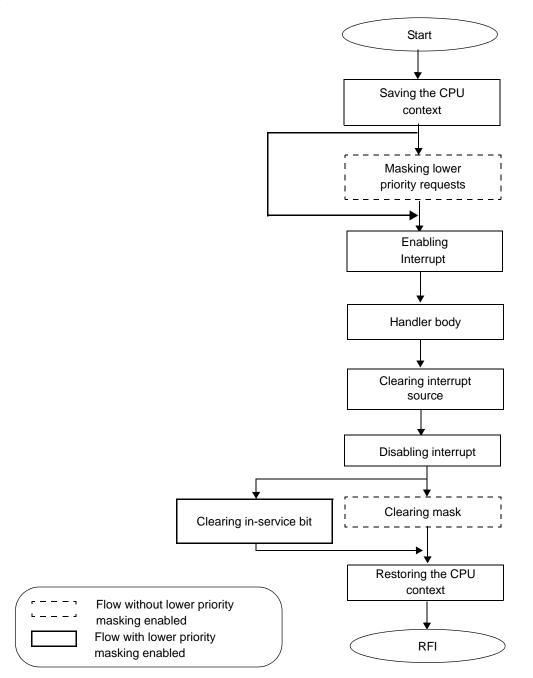
Figure 6-6. Typical Interrupt Handler Routine
