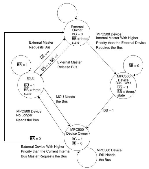
Figure 9-27. Internal Bus Arbitration State Machine
