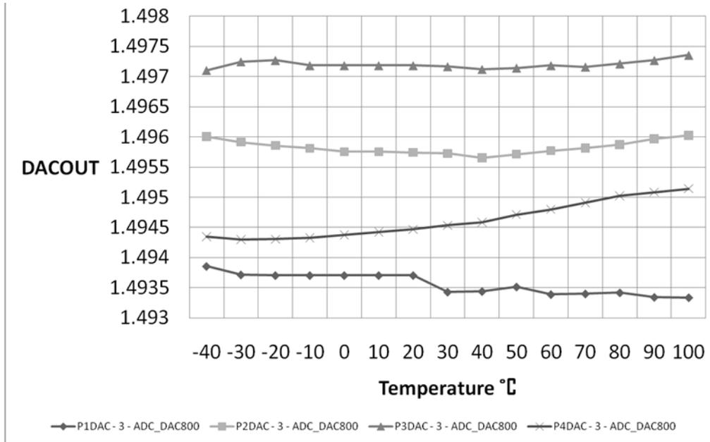
Figure 7. Offset at Half Scale vs Temperature
