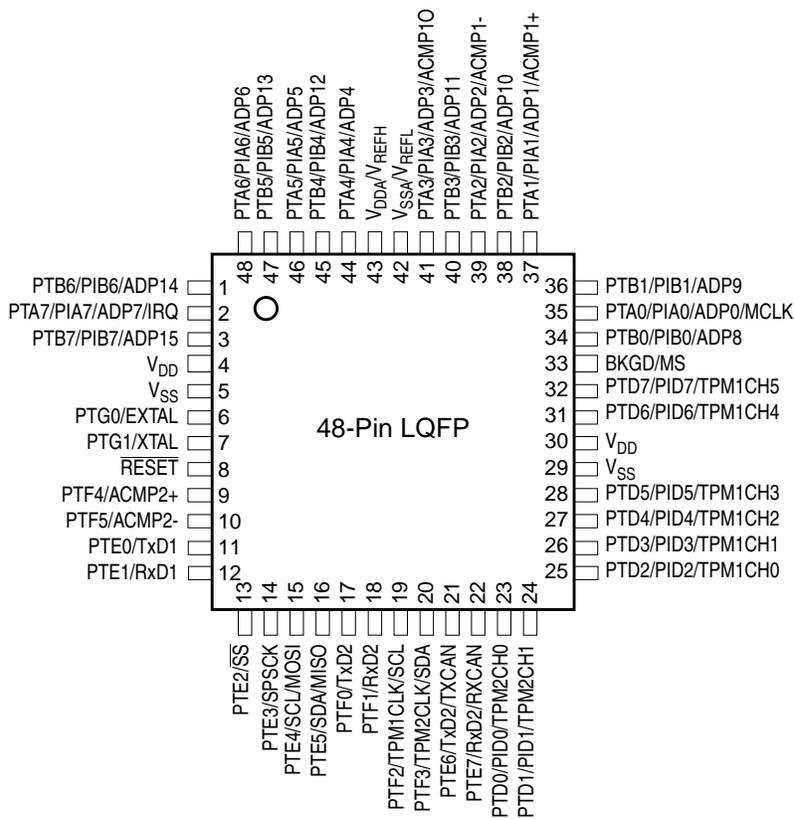
V<sub>REFH</sub> and V<sub>REFL</sub> are internally connected to V<sub>DDA</sub> and V<sub>SSA</sub>, respectively.
