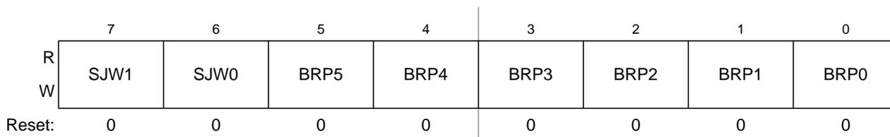
**Figure 12-6. MSCAN Bus Timing Register 0 (CANBTR0)**
