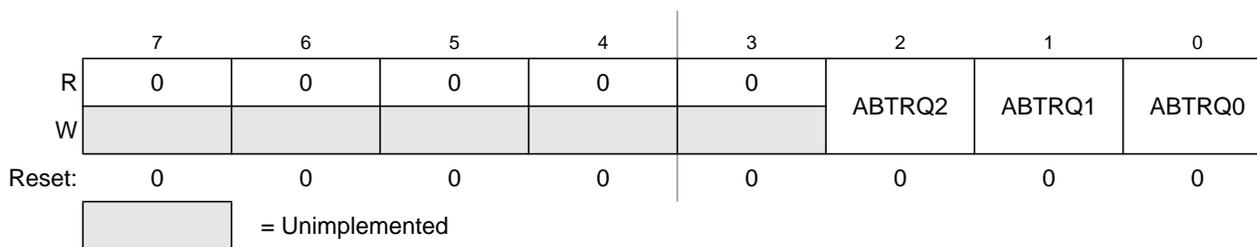
**Figure 12-12. MSCAN Transmitter Message Abort Request Register (CANTARQ)**
