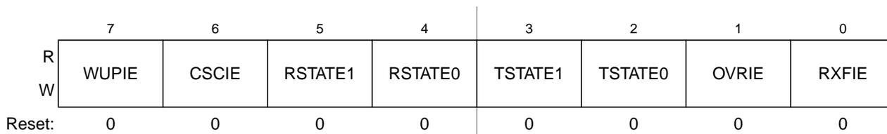
**Figure 12-9. MSCAN Receiver Interrupt Enable Register (CANRIER)**
