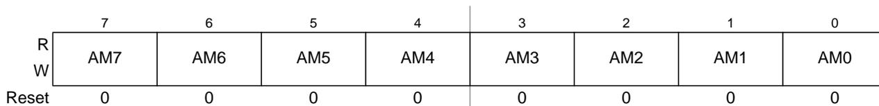
**Figure 12-22. MSCAN Identifier Mask Registers (Second Bank) — CANIDMR4–CANIDMR7**
