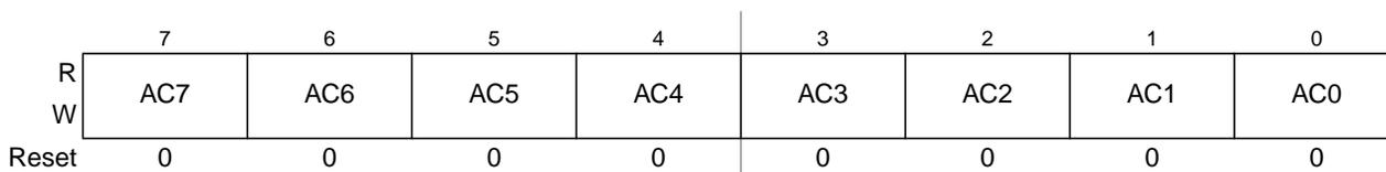
**Figure 12-19. MSCAN Identifier Acceptance Registers (First Bank) — CANIDAR0–CANIDAR3**
