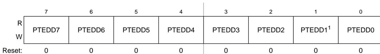
**Figure 6-33. Port E Data Direction Register (PTEDD)**
