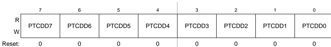
Figure 6-20. Port C Data Direction Register (PTCDD)
