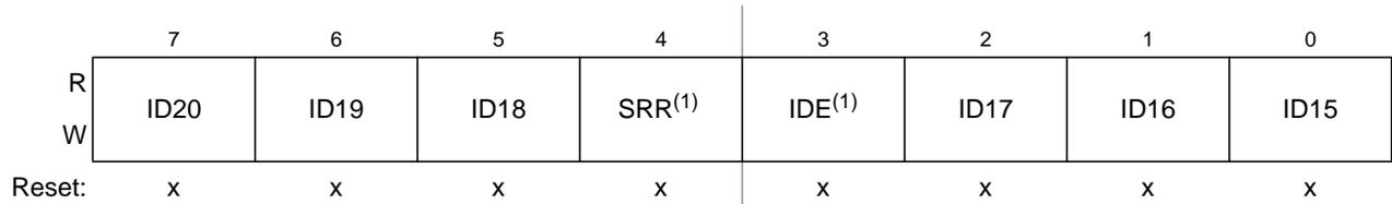
**Figure 12-26. Identifier Register 1 (IDR1) — Extended Identifier Mapping**
