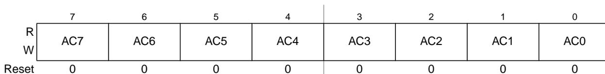
**Figure 12-20. MSCAN Identifier Acceptance Registers (Second Bank) — CANIDAR4–CANIDAR7**
