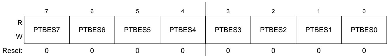
Figure 6-18. Port B Edge Select Register (PTBES)
