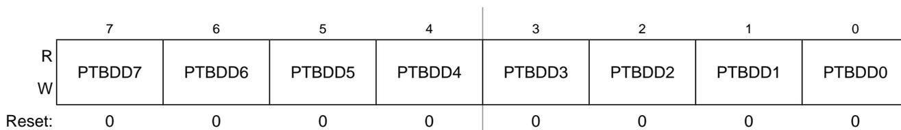
Figure 6-12. Port B Data Direction Register (PTBDD)
