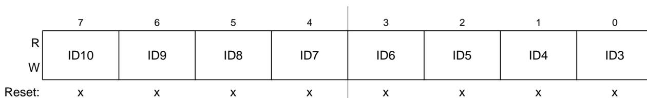
Figure 12-29. Identifier Register 0 — Standard Mapping
