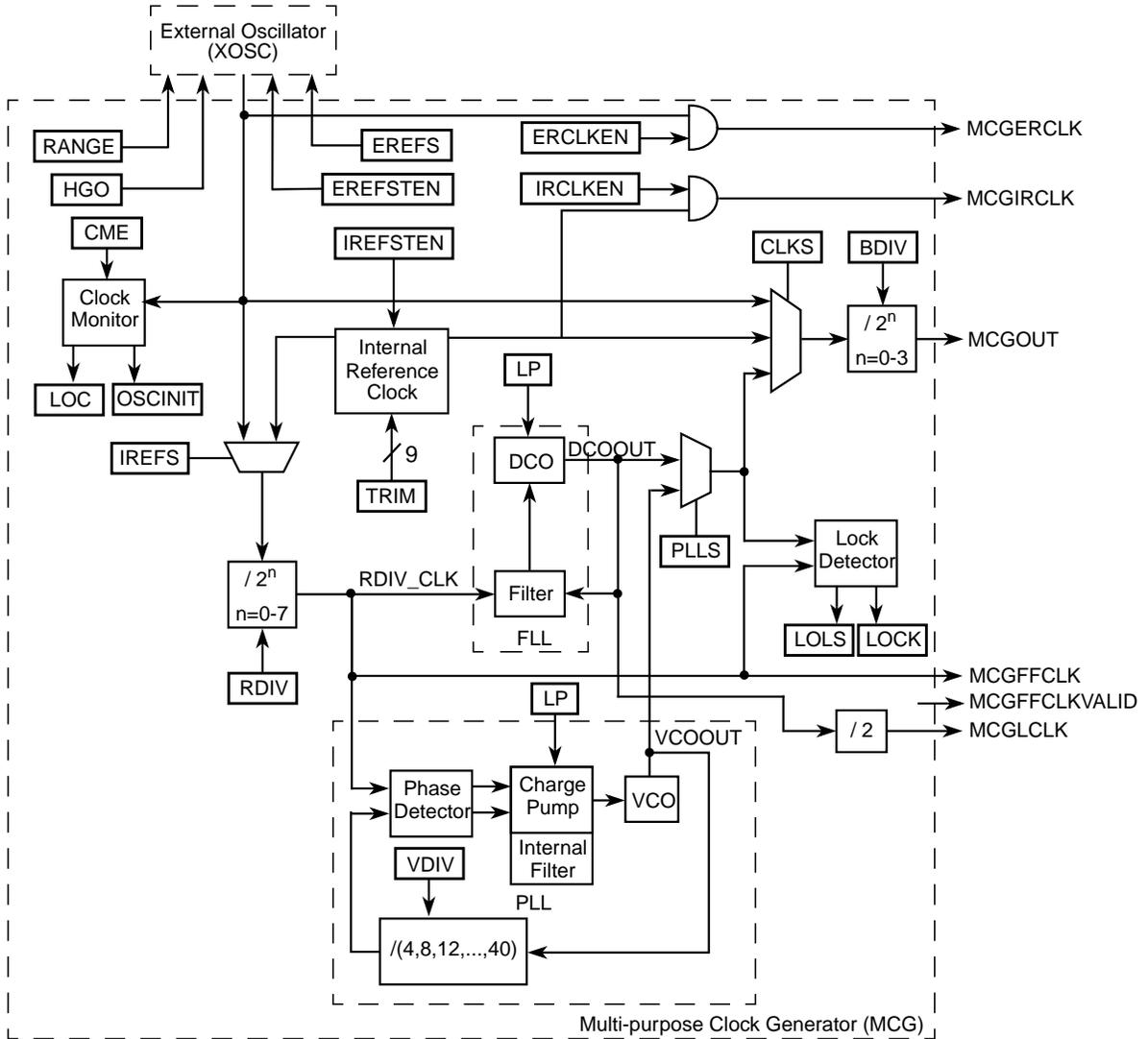
Figure 8-2. Multi-Purpose Clock Generator (MCG) Block Diagram
