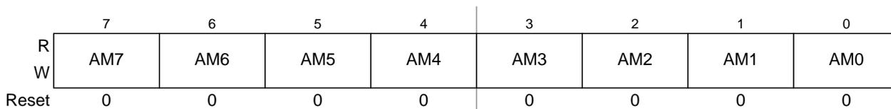
**Figure 12-21. MSCAN Identifier Mask Registers (First Bank) — CANIDMR0–CANIDMR3**
