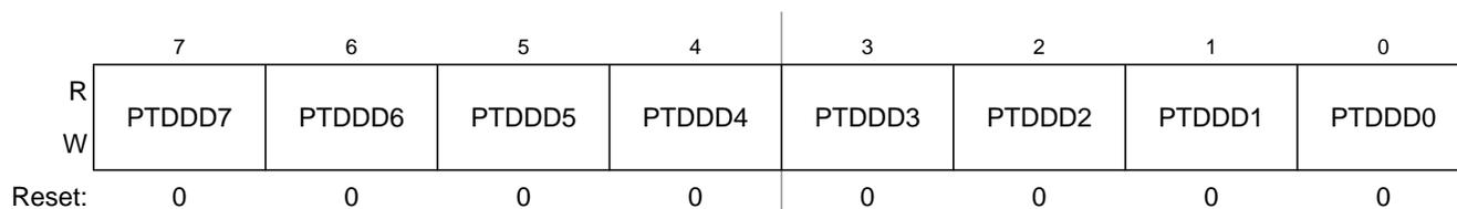
Figure 6-25. Port D Data Direction Register (PTDDD)
