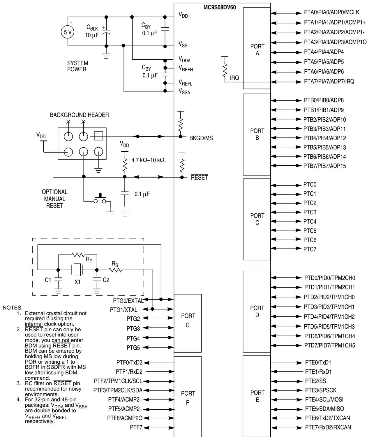
Figure 2-4. Basic System Connections (Shown in 64-Pin Package)
