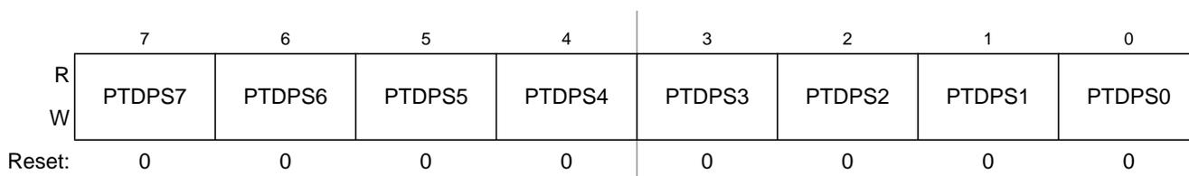
Figure 6-30. Port D Interrupt Pin Select Register (PTDPS)
