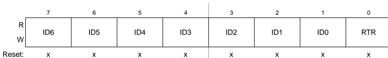
Figure 12-28. Identifier Register 3 (IDR3) — Extended Identifier Mapping
