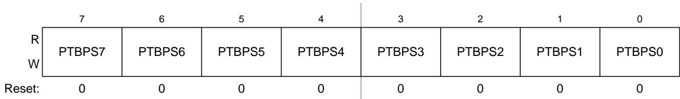
Figure 6-17. Port B Interrupt Pin Select Register (PTBPS)
