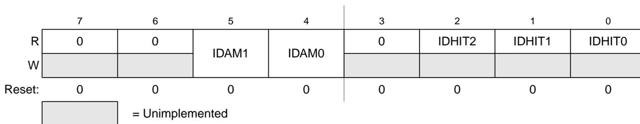
**Figure 12-15. MSCAN Identifier Acceptance Control Register (CANIDAC)**
