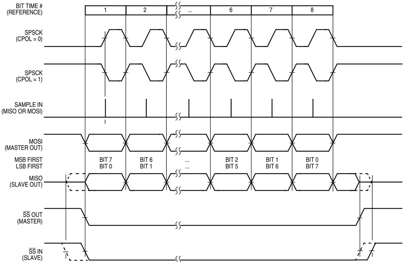
Figure 13-11. SPI Clock Formats (CPHA = 0)
