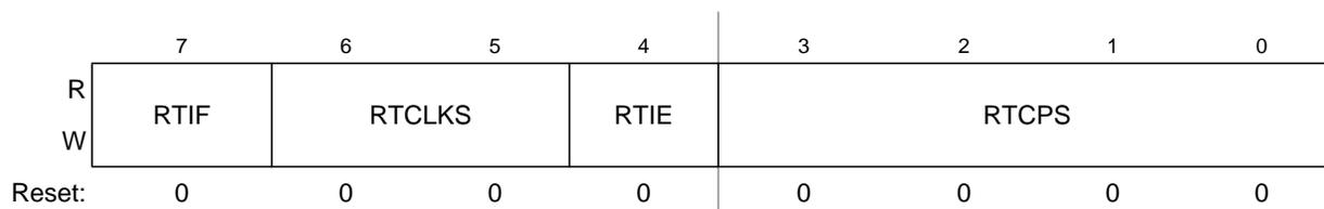
**Figure 15-3. RTC Status and Control Register (RTCSC)**
