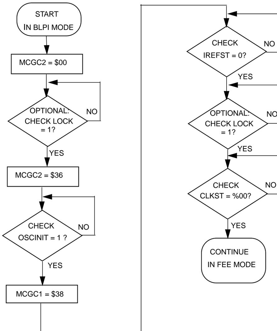
Figure 8-11. Flowchart of BLPI to FEE Mode Transition using a 4 MHz crystal
