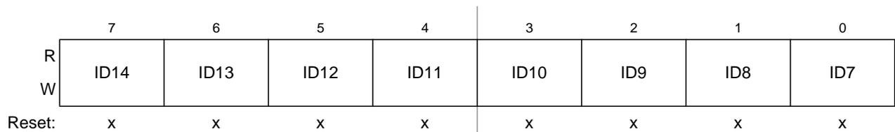
**Figure 12-27. Identifier Register 2 (IDR2) — Extended Identifier Mapping**
