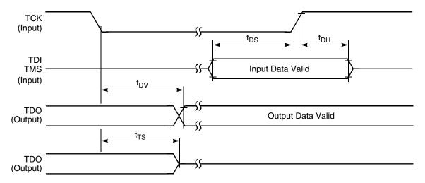
Figure 8. Test access port timing diagram
