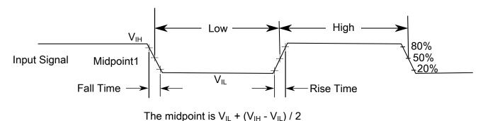
Figure 5. Input signal measurement references
