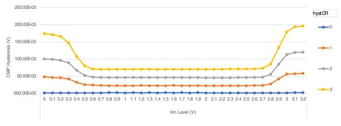
Figure 12. Typical hysteresis vs. Vin level ( $V_{DD} = 3.3 \text{ V}$ , PMODE = 0)
