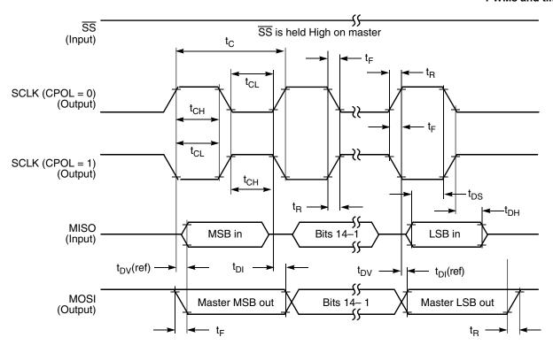
Figure 17. SPI master timing (CPHA = 1)
