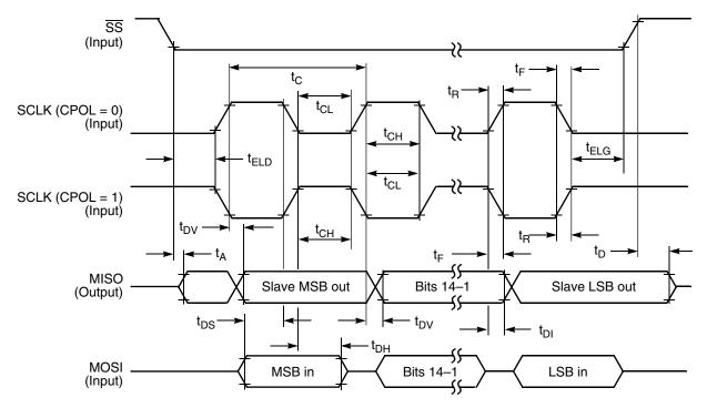
Figure 19. SPI slave timing (CPHA = 1)
