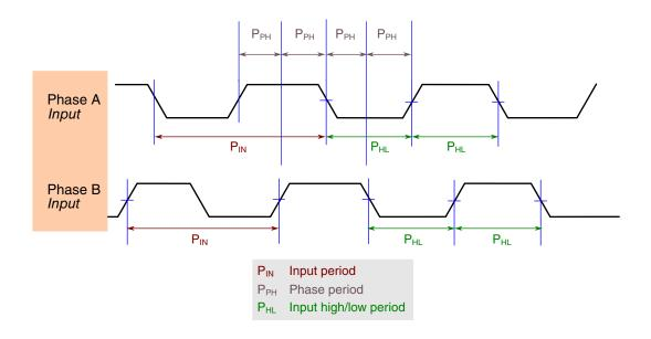
Figure 15. Quadrature Decoder Timing
