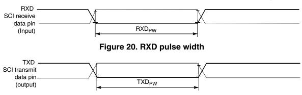
Figure 21. TXD pulse width
