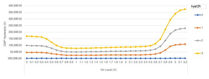
Figure 13. Typical hysteresis vs. Vin level ( $V_{DD} = 3.3 \text{ V}$ , PMODE = 1)
