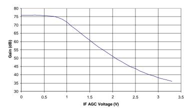
Figure 32. Tuner Gain versus IF AGC Voltage
