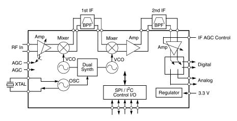
Figure 1. MC44S803 Functional Block Diagram
