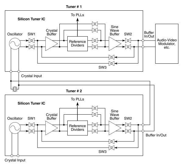
Figure 34. Two Receivers and Modulator Sharing One Crystal
