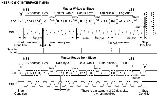
Figure 6. I<sup>2</sup>C Timing Diagram
