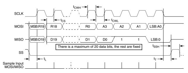
Figure 5. SPI Timing Diagram
