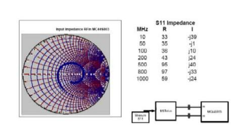
RFinput Impedance and Measurement Circuit
