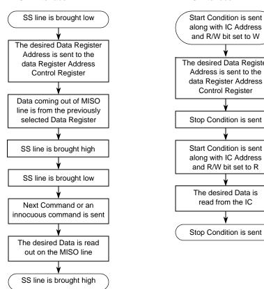
is both a read and a write operation. But the data being read out is not affected by the command that is actively being written to the IC. The command doesn't take effect until the SPI operation is completed.
