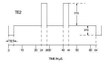
Figure 8. Test Pattern Generator
