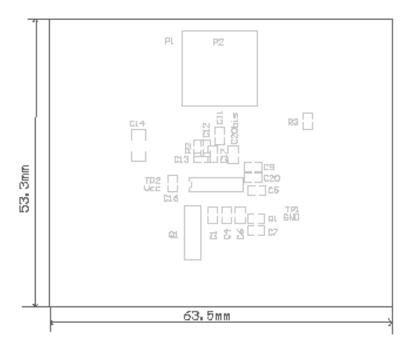
Figure 15. Evaluation Board PCB Layout
