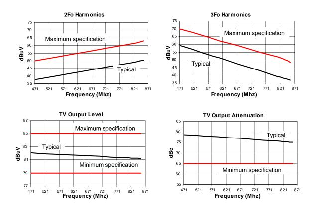
Figure 3. Typical High Frequency Performance
