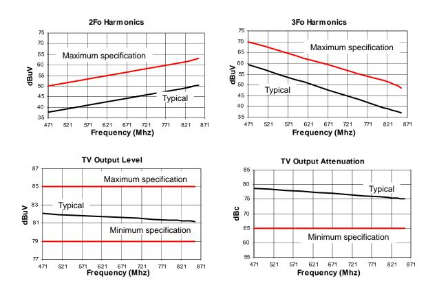
Figure 4. Typical High Frequency Performance
