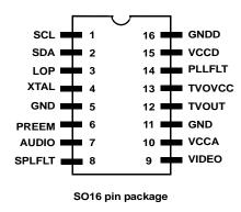
Figure 1. MC44BS374T1 and MC44BS374T1A Pin Connections
