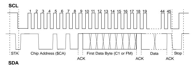
Figure 12. I<sup>2</sup>C Bus Timing
