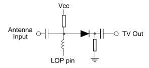
Figure 7. Typical Attenuator Application with Pin Diode
