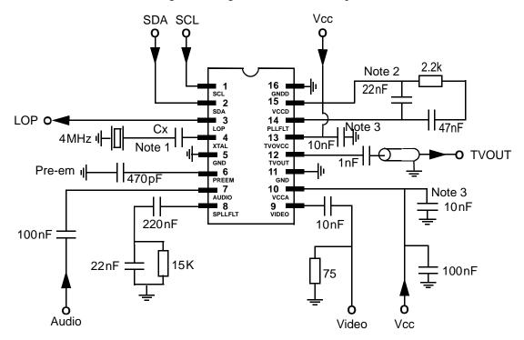
Figure 14. Proposed Application Schematic
