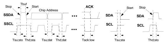
Figure 10. SSDA/SSCL Timing
