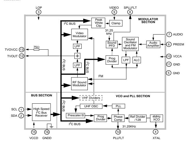
Figure 2. MC44BS374T1/374T1A Simplified Block Diagram
