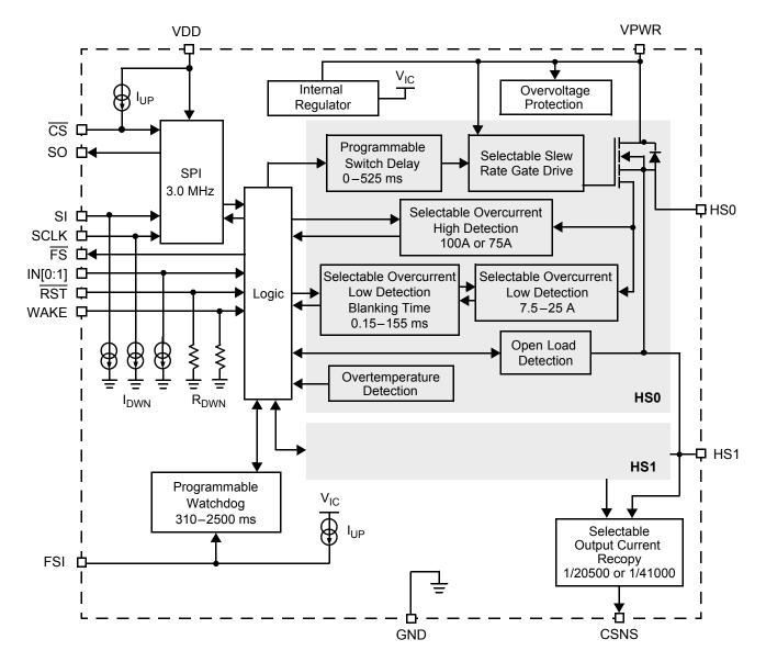
Figure 2. 34984 Simplified Internal Block Diagram
