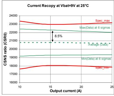
Figure 15. CSR0 Ratio Deviation in Function Manufacturing
