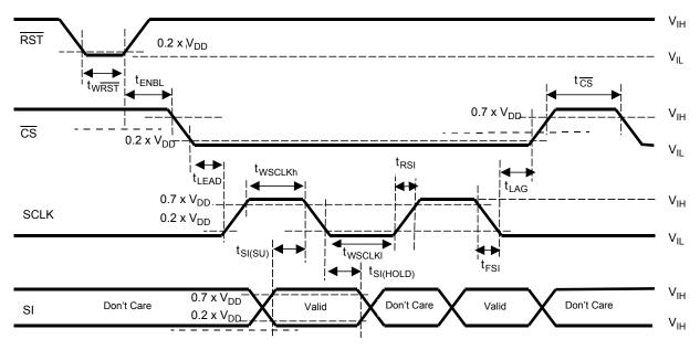
Figure 7. Input Timing Switching Characteristics
