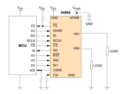
Figure 1. 34984 Simplified Application Diagram
