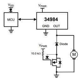
Figure 9. Reverse Voltage Protection
