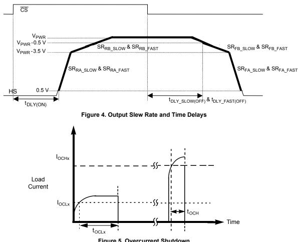
Figure 5. Overcurrent Shutdown
