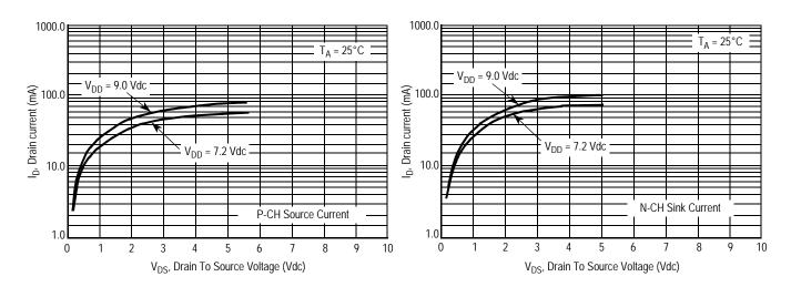
Figure 5. Typical P Horn Driver Output I-V Characteristic
