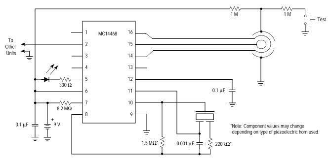
Figure 6. Typical Application as Ionization Smoke Detector
