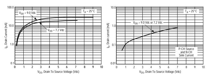
Figure 3. Typical LED Output I-V Characteristic
