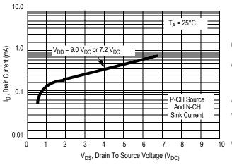
Figure 4. Typical Comparator Output I-V Characteristic
