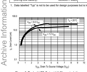
Figure 3. Typical LED Output I-V Characteristic
