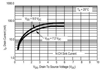
Figure 5. Typical P Horn Driver Output I-V Characteristic
