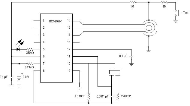
\*NOTE: Component values may change depending on type of piezoelectric horn used.
