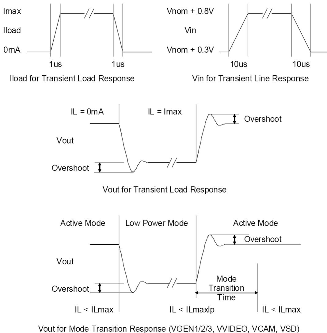
**Figure 25. Transient Waveforms**
