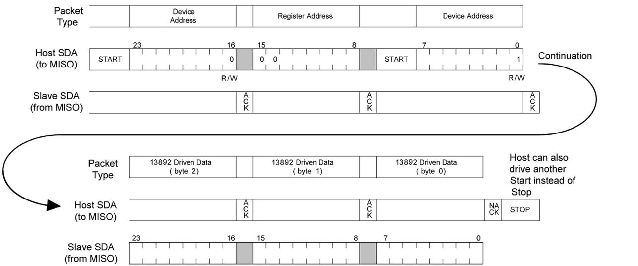
Figure 9. I<sup>2</sup>C 3 Byte Read Example
