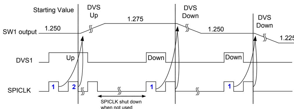
**Figure 21. SID Control Example for Increment & Decrement**
