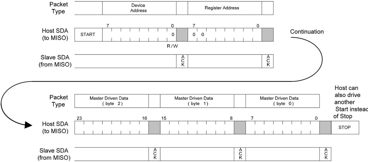
Figure 8. I<sup>2</sup>C 3 Byte Write Example
