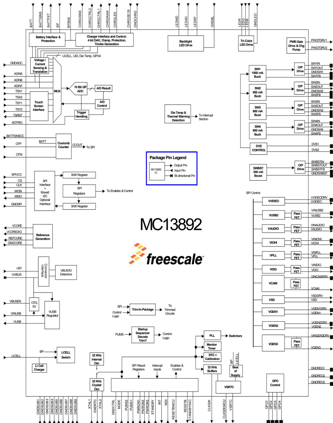
Figure 2. MC13892 Simplified Internal Block Diagram
