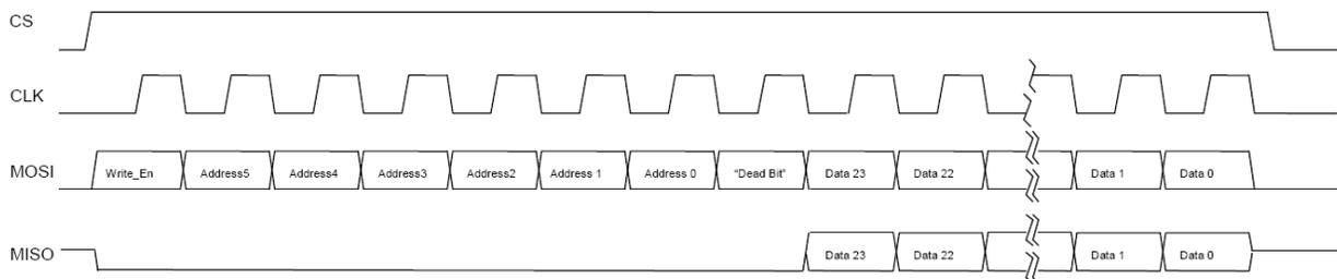
**Figure 5. SPI Transfer Protocol Single Read/Write Access**
