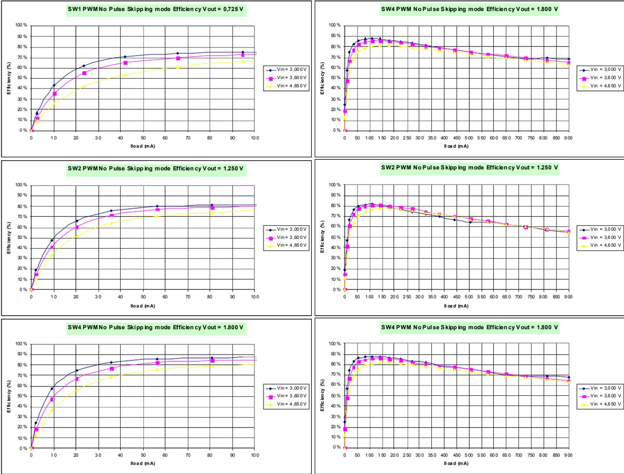
Figure 18. Buck Regulator PWM (No Pulse Skipping) Efficiency
