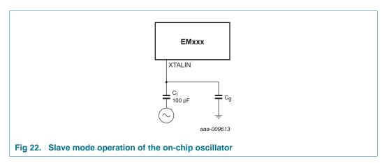
In slave mode, the input clock signal should be coupled using a capacitor of 100 pF (Figure 22), with an amplitude between 200 mV (RMS) and 1000 mV (RMS). This corresponds to a square wave signal with a signal swing of between 280 mV and 1.4 V. The XTALOUT pin in this configuration can be left unconnected.
