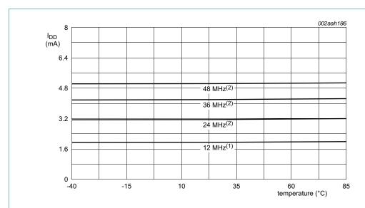
Conditions:  $V_{DD(3V3)} = 3.3 \text{ V}$ ; sleep mode entered from flash; all peripherals disabled in the SYSAHBCLKCTRL register and PDRUNCFG register; all peripheral clocks disabled; BOD disabled; power mode 0 (see Section 7.18.6.2).
