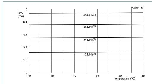
Conditions:  $V_{DD(3V3)} = 3.3 \text{ V}$ ; active mode entered executing code while (1) {} from flash; all peripherals disabled in the SYSAHBCLKCTRL register; all peripheral clocks disabled; all analog peripherals disabled in the PDRUNCFG register; power mode 0 (see Section 7.18.6.2).
