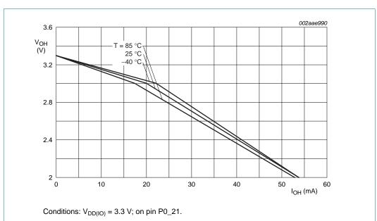
Fig 8. High-current source output driver: Typical HIGH-level output voltage V<sub>OH</sub> versus HIGH-level output current I<sub>OH</sub>
