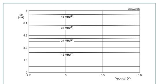
Conditions:  $V_{DD(3V3)} = 3.3 \text{ V}$ ; active mode entered executing code while(1){} from flash; all peripherals enabled in the SYSAHBCLKCTRL register; all analog peripherals enabled in the PDRUNCFG register; power mode 0 (see Section 7.18.6.2).
