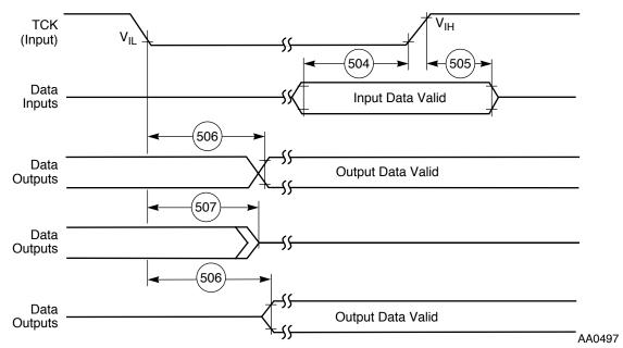
Figure 2-12 Boundary Scan (JTAG) Timing Diagram
