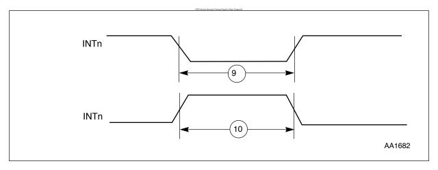
Figure 2-4 INT0–INT7 External Interrupt Timing
