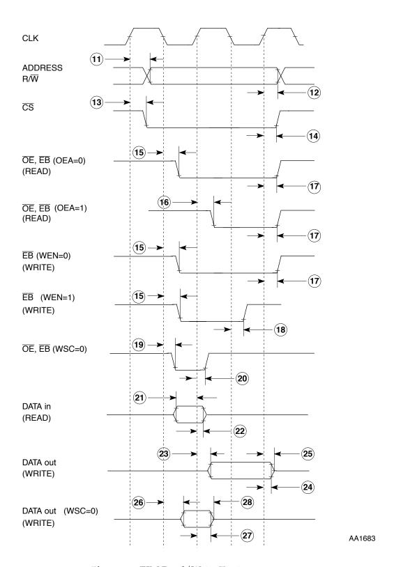
Figure 2-5 EIM Read/Write Timing
