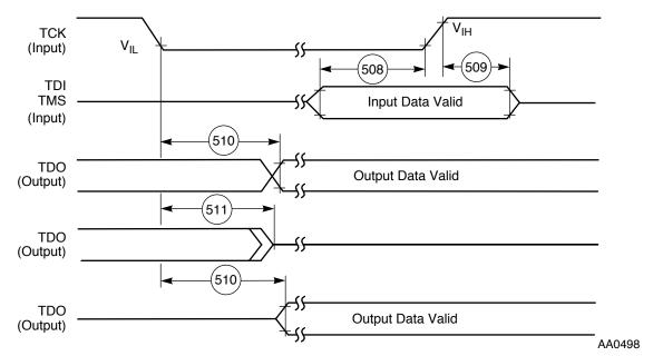
Figure 2-14 Test Access Port Timing Diagram
