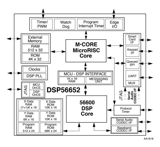
Figure 1-1 DSP56652 System Block Diagram
