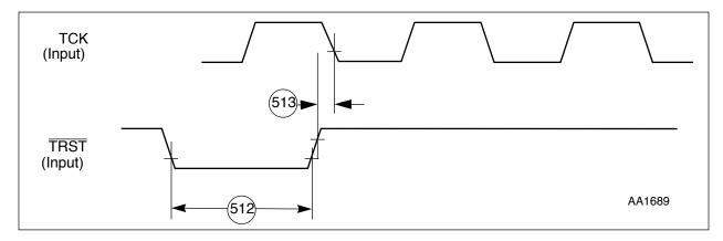
Figure 2-13 TRST Timing Diagram
