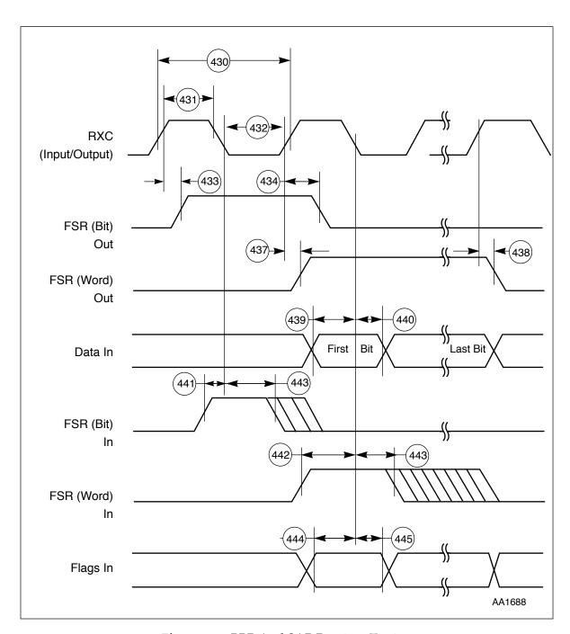
Figure 2-10 BBP And SAP Receiver Timing
