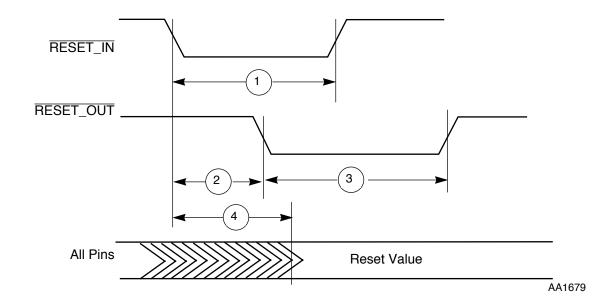
Figure 2-1 Reset Timing
