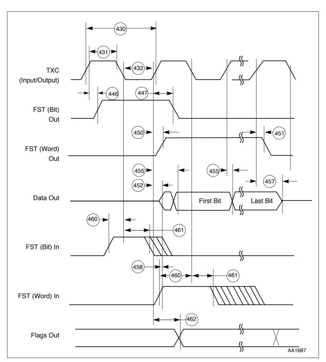
**Note:** In the network mode, output flag transitions can occur at the start of each time slot within the frame. In the normal mode, the output flag state is asserted for the entire frame period.
