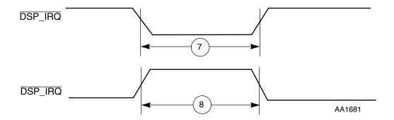
Figure 2-3 DSP External Interrupt Timing (Negative Edge-Triggered)
