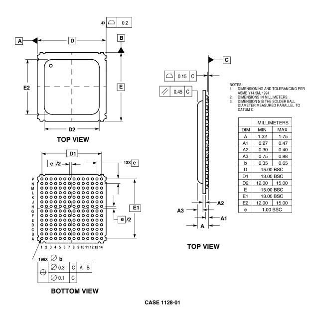
Figure 3-1 DSP56652 Mechanical Information, 196-pin PBGA Package
