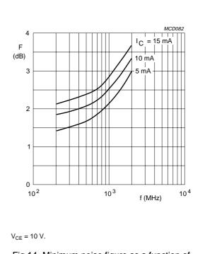
Fig.14 Minimum noise figure as a function of frequency; typical values.
