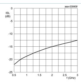
Diode zero-biased and inserted in series with a 50  $\Omega$  strip line circuit and biased via the analyzer T-network;  $T_{amb}$  = 25 °C; f = 100 MHz
