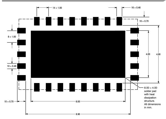
Figure 3. PCB Pad Layout for 10 mm  $\times$  6 mm Module
