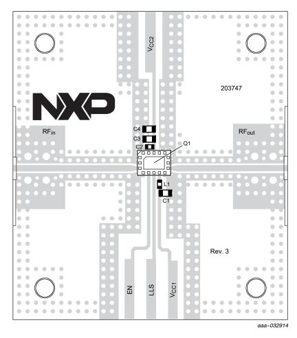
Figure 3. AFLP5G35645 Application Circuit Component Layout
