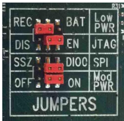
Figure 2: DR1174 JTAG Jumper Position
