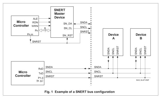
The data transmitted or received is made up of address and data bytes alternatively. A SNERT message can consist of one or more pairs of address and data bytes. The address/data sequence is
