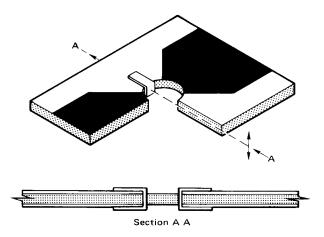
Figure 6. Proper Emitter Grounding Method
