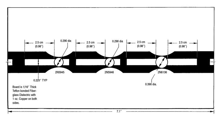
Figure 7. Microstrip Board Layout
