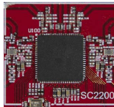
Figure 4. SC2200 RFPAL Layout Showing External PCB Components
