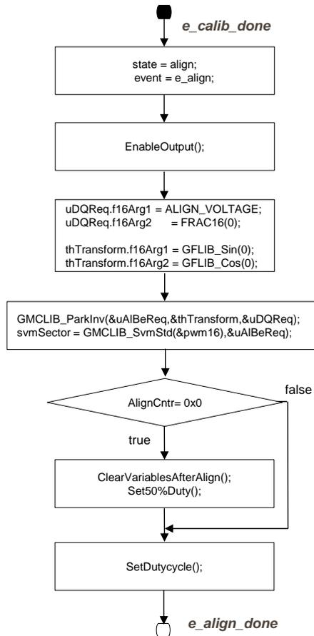
Figure 22. Flow chart of state ALIGN
