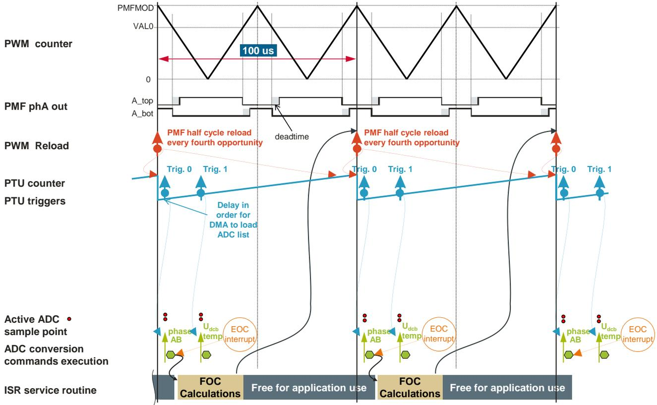
Figure 10. Time Diagram of PWM and ADC Synchronization
