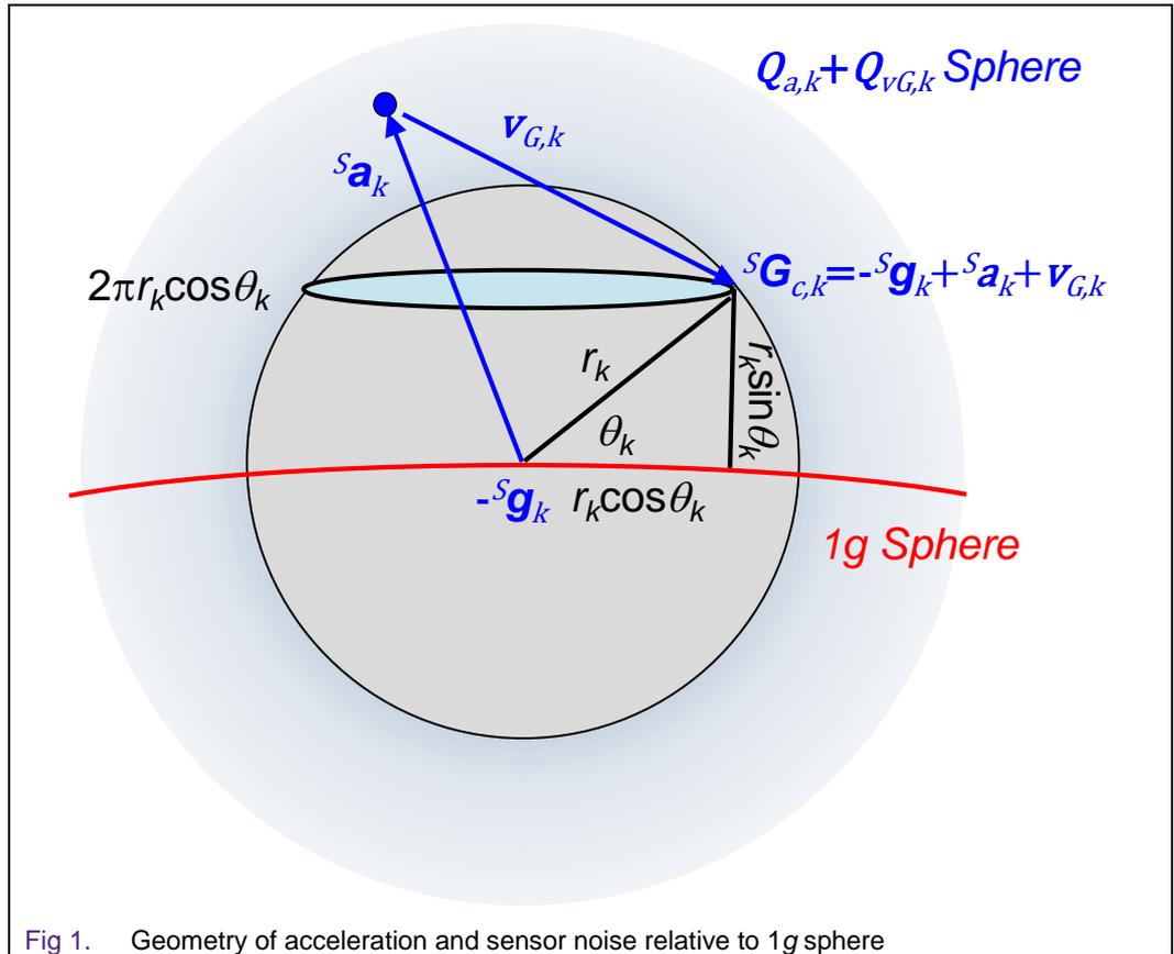
Fig 1. Geometry of acceleration and sensor noise relative to 1g sphere
