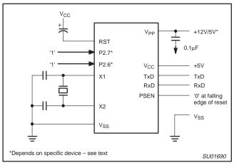
Figure 1. In-System Programming with a Minimum of Pins
