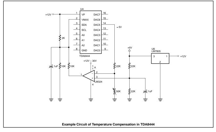
All VRs in this application note can be charged to fix resistors, when proper dividing voltage is determined.
