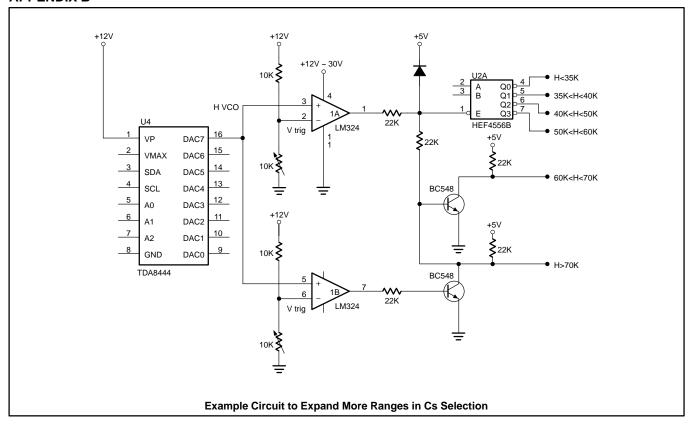
When you want to determine Vtrig signal, please disconnect Pulse Signal Generator (P.S.G.) Output to H. Sync demoboard from monitor and connect, and use input, set P.S.G. to 60kHz, TTL level output, then power on the demoboard, the mode display should display "19", the the voltage in DAC H-V output pin is the trigger level voltage of 60kHz. You can set P.S.G to 70kHz to measure trigger level voltage of 70kHz.
