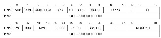
**Figure 1. Hard Reset Configuration Word**
